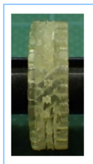
Figure 5 Coil holder fabricated using AM technology
