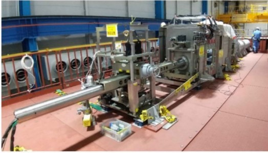
Testing of fuel debris trial retrieval device with mockups
