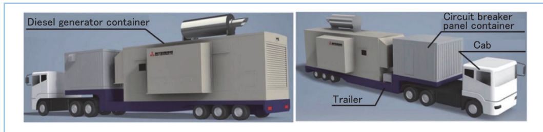
Figure 7 Structure of onboard air-cooled DG
