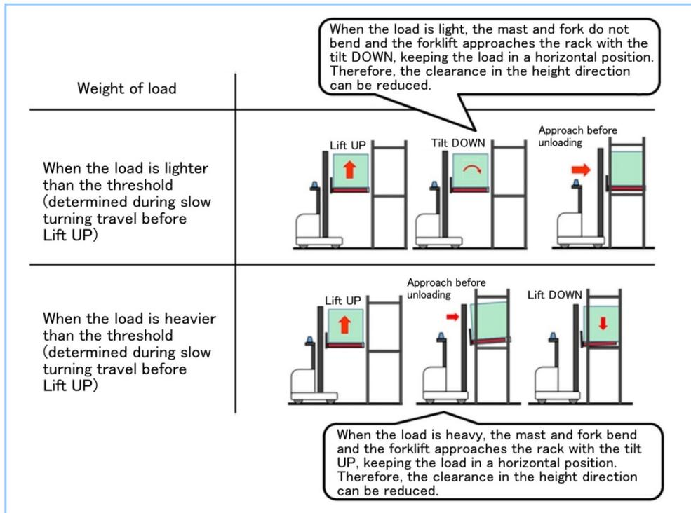
**Figure 2 Unloading operation flow of improved performance AGF**
