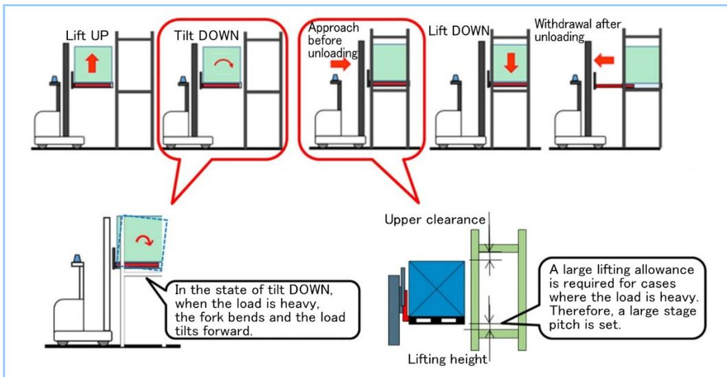
**Figure 1 Unloading operation flow of conventional model**
