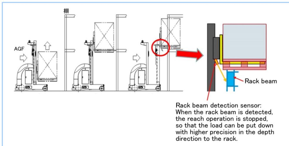
**Figure 3 Rack beam detection mechanism**
