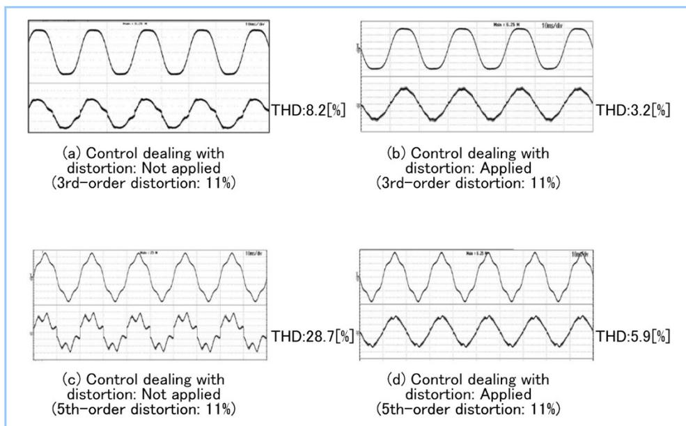
Figure 6 Measured waveform
