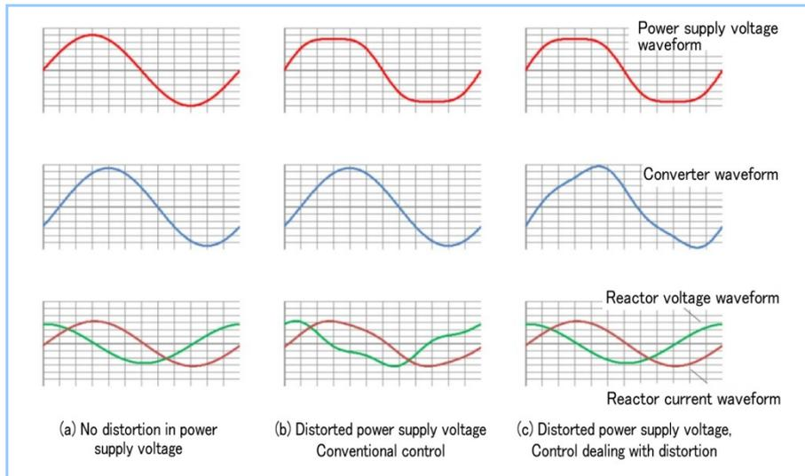
**Figure 2 Converter that deals with distorted power supply voltage**
