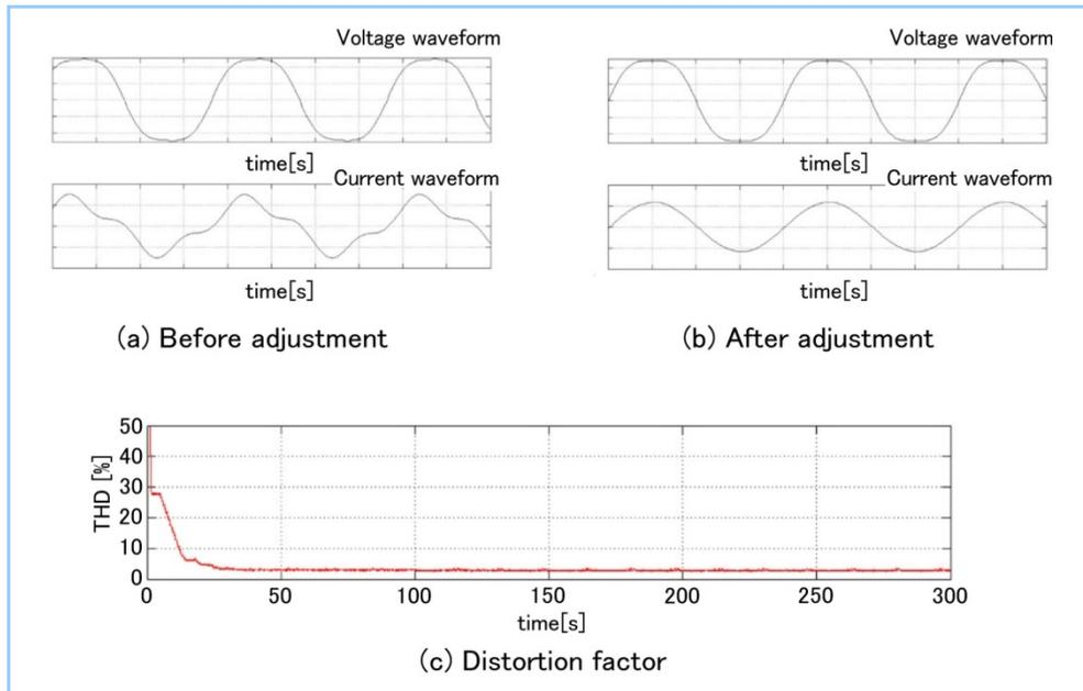
Figure 5 Simulation waveform
