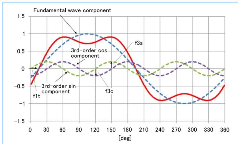
Figure 3 Converter waveform (superimposed with harmonics)
