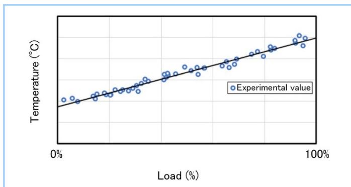
**Figure 8 Measurement results of internal gear temperature**
