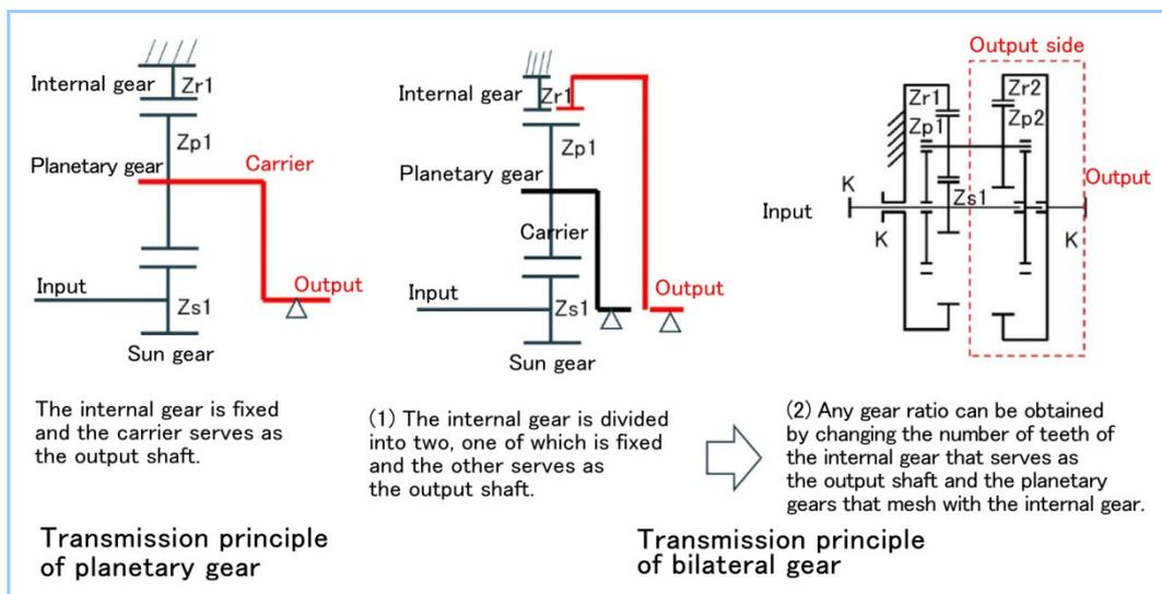
**Figure 2 Comparison of transmission principles of bilateral gear and conventional planetary gear**
