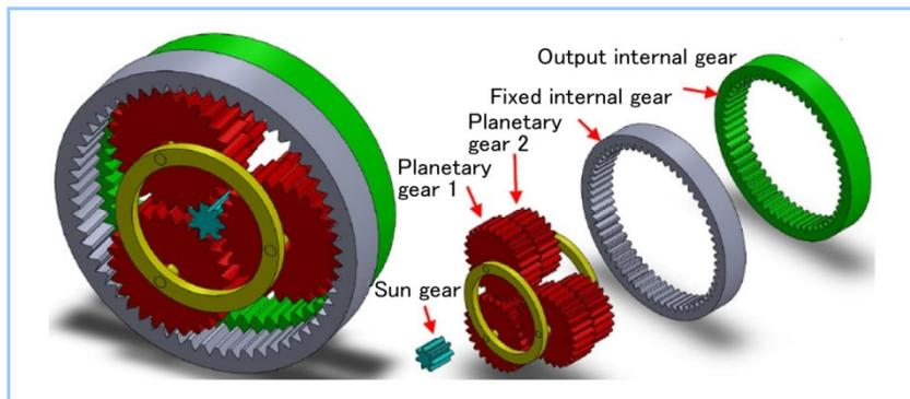
**Figure 1 Structure of bilateral gear**
