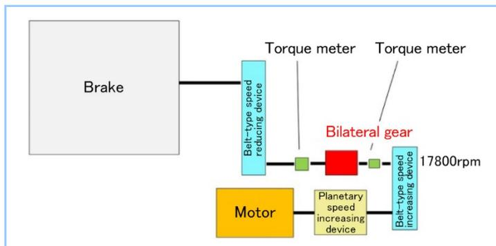
**Figure 6 Configuration of bilateral gear load test equipment**
