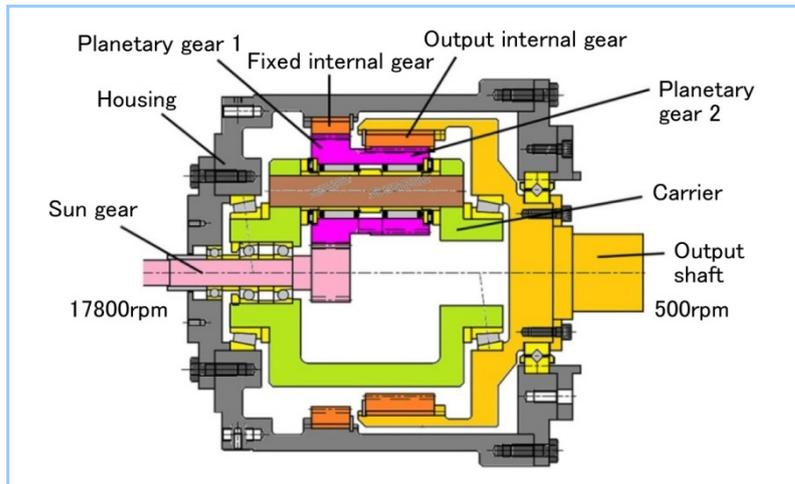
**Figure 5 Structure of prototype bilateral gear**
