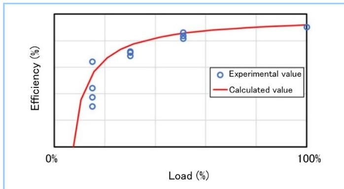
**Figure 7 Measurement results of bilateral gear efficiency**
