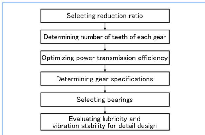
**Figure 3 Design procedure of bilateral gear**
