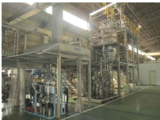
**Figure 5 Biomass gasification and FT synthesis integration test facility**
