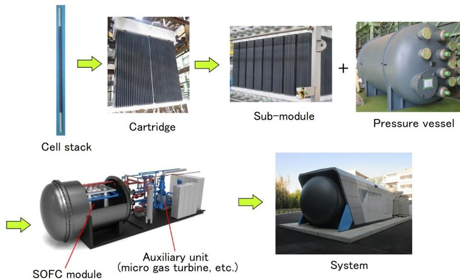
**Figure 2** Composition of hybrid system
