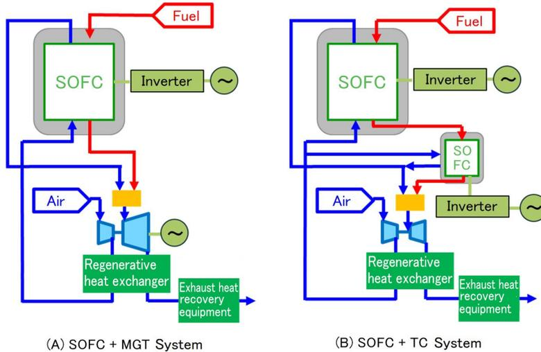
Figure 3 Comparison of MGT system and TC system
