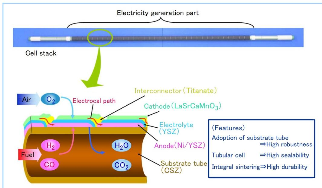
**Figure 1** Structure of cell stack
