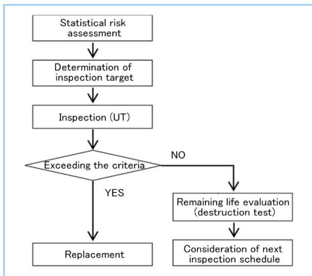
**Figure 10** Conceptual diagram of maintenance flow against failure on weld interface of low alloy steel dissimilar welds
