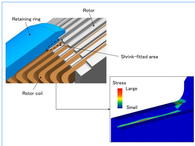
**Figure 8** Stress analysis of rotor end
