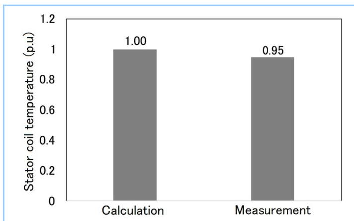
**Figure 10** Comparison of measured maximum temperature and calculation result of stator coil
