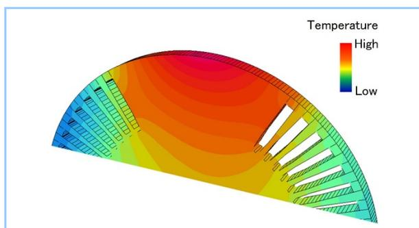
**Figure 9** Analysis of rotor body temperature in thyristor starting
