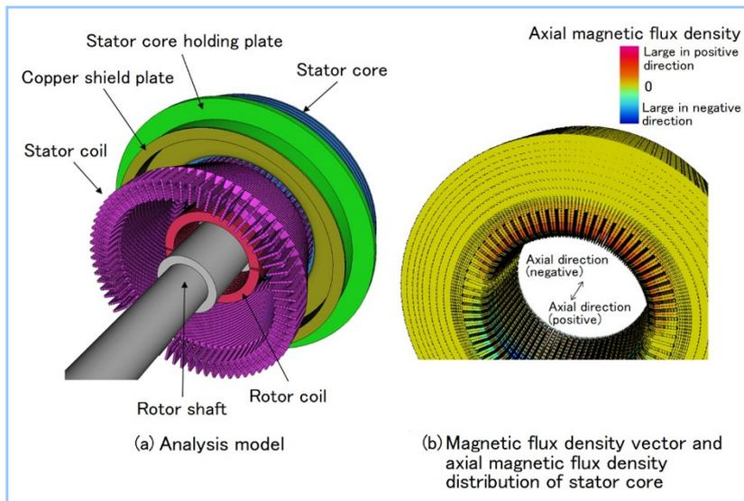
**Figure 6** Magnetic field analysis of stator core end
