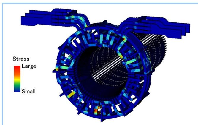
**Figure 7** Electromagnetic force-vibration response analysis of stator coil end
