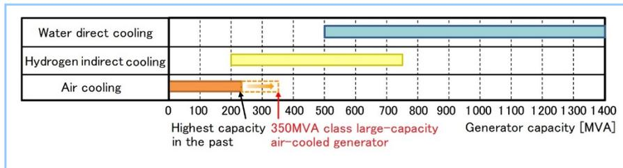
Figure 1 Relationship between stator coil cooling method and generator capacity
