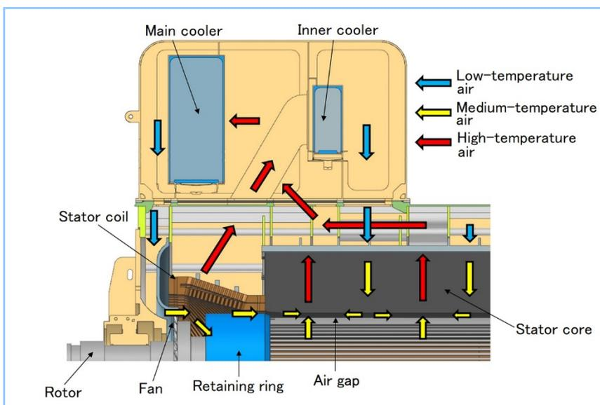
**Figure 5** Inner cooler airflow circuit
