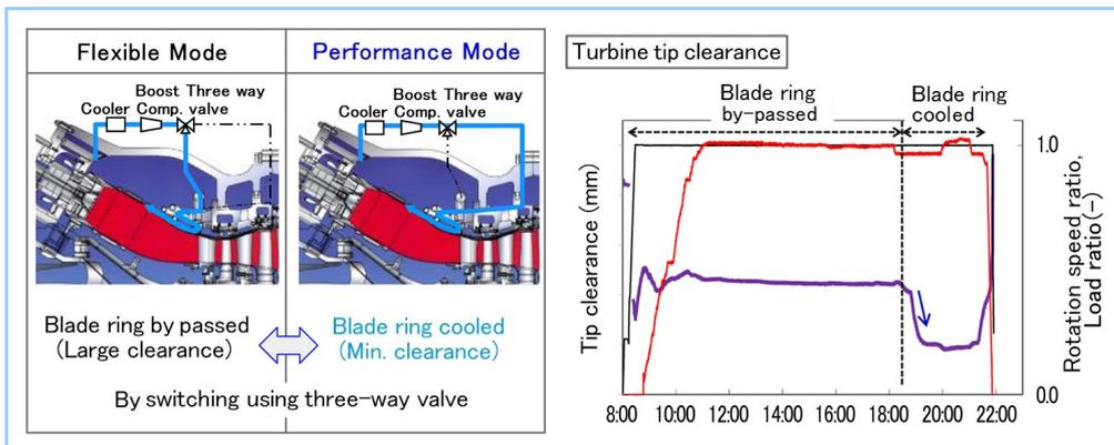
Figure 8 Turbine clearance control using enhanced air-cooled system
