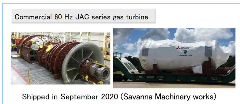
**Figure 13 Shipping of commercial 60 Hz M501JAC gas turbine**
