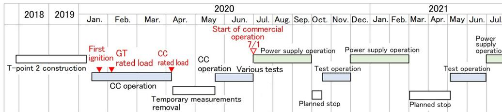
**Figure 4 Test operation schedule at T-point 2**
