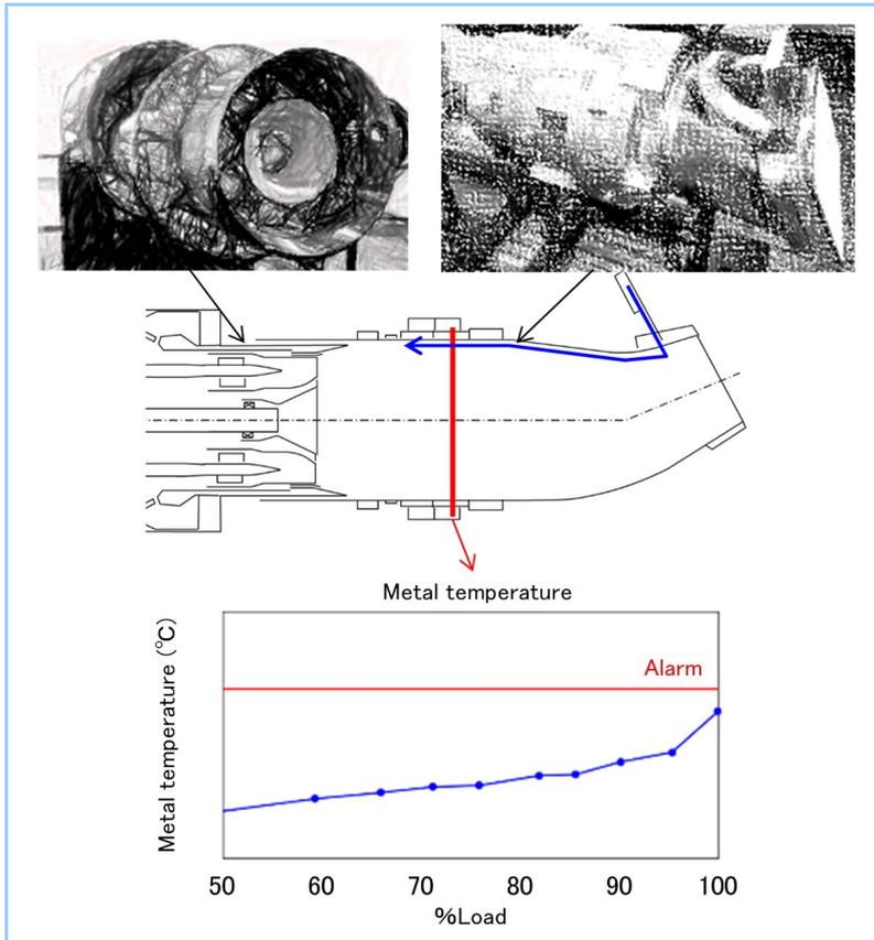
Figure 7 Measurement results of enhanced air-cooled combustor metal temperature
