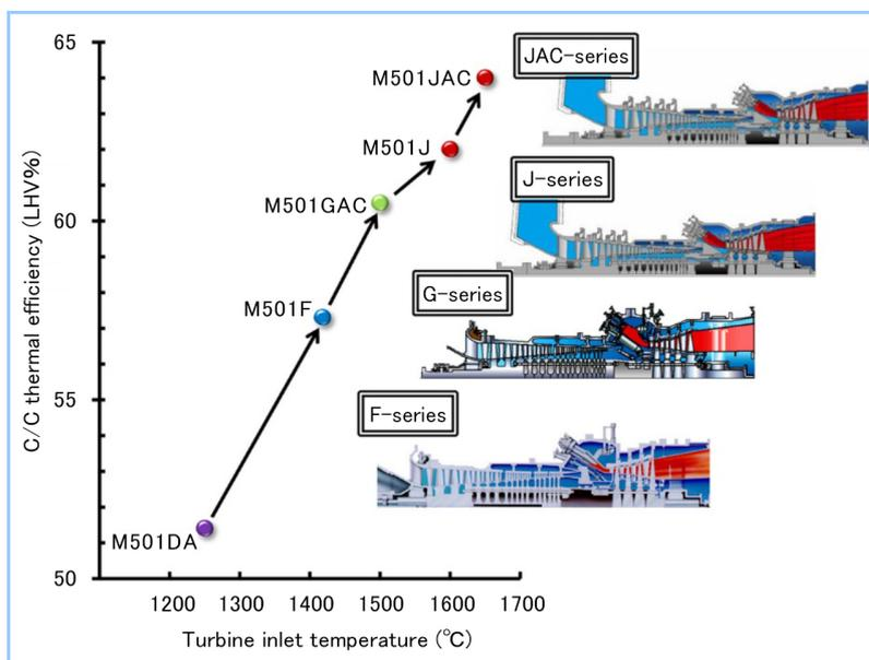
Figure 1 Developmental trend of large gas turbine models
