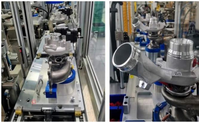
**Figure 2** Locally-procured turbocharger assembly line
