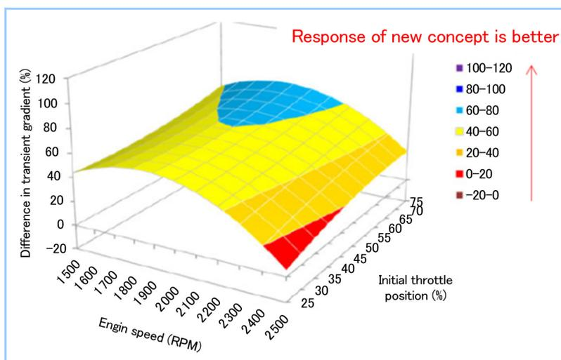
Figure 9 Comparison of engine response between conventional compressor and new concept compressor
