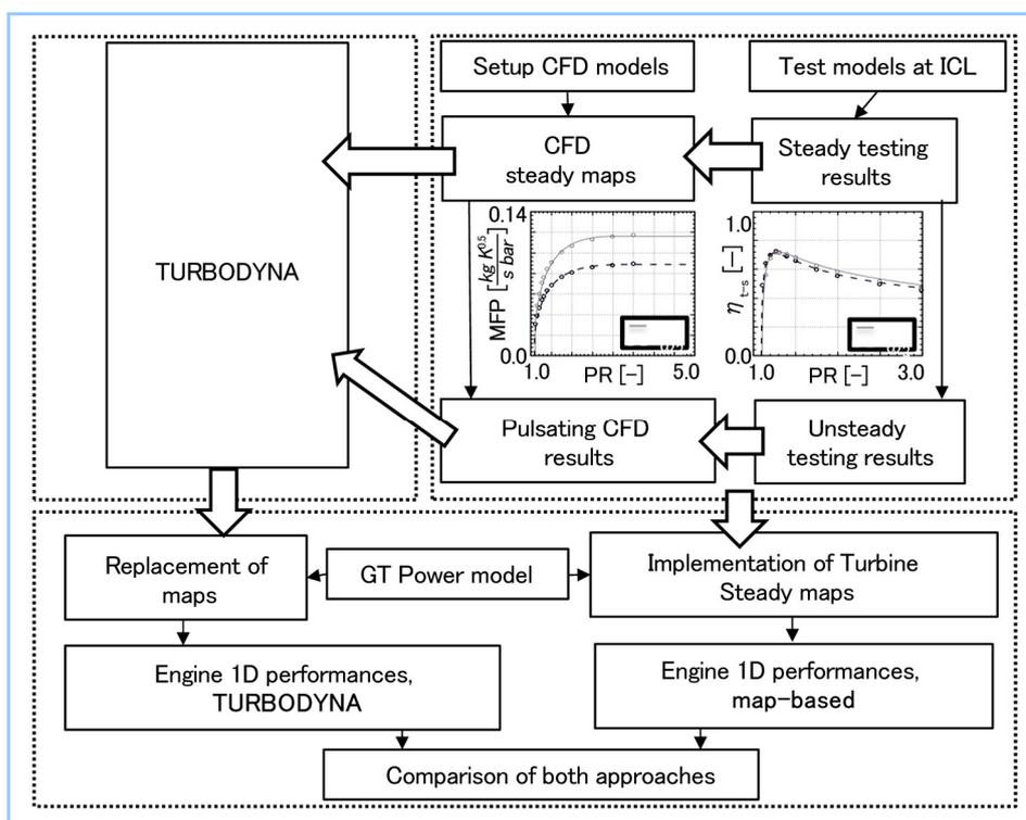
**Figure 11** Development flow of engine performance evaluation method considering turbine unsteady performance
