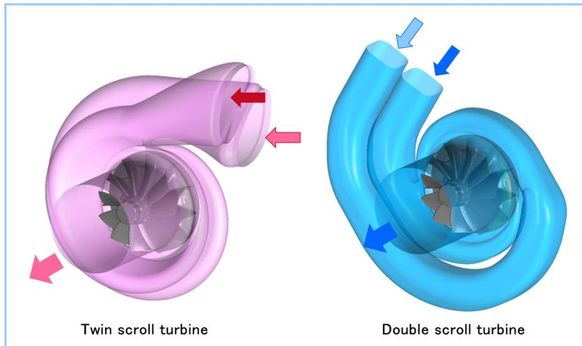
**Figure 12 Comparison of double entry turbines structures**
