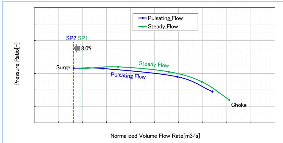
Figure 4 Relationship between presence of pressure pulsation and surge flow rate
