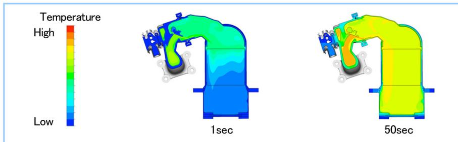
**Figure 10** Unsteady turbine CHT (Conjugate Heat Transfer) analysis result at cold start
