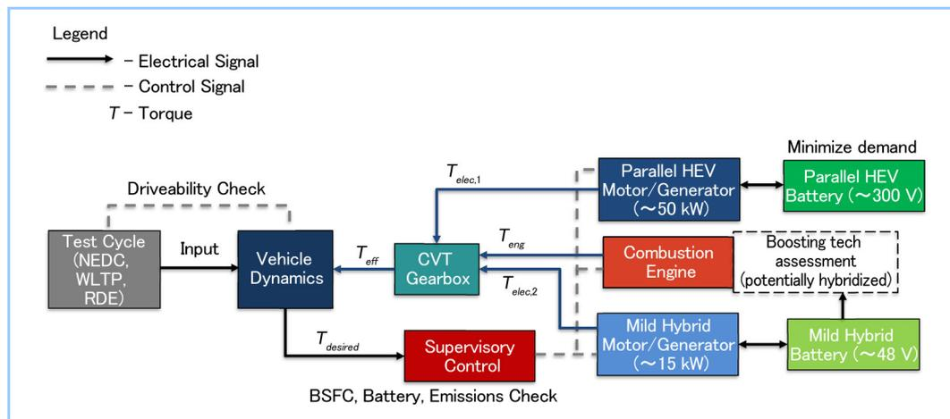
Figure 14 Structure of vehicle system model for hybrid vehicle
