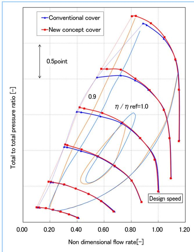
Figure 7 Compressor performance test result
