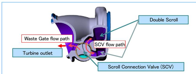
**Figure 13 Cross-Sectional view of double scroll turbine SCV and functional description**
