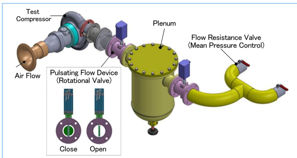
**Figure 3** Compressor pulsating flow test equipment
