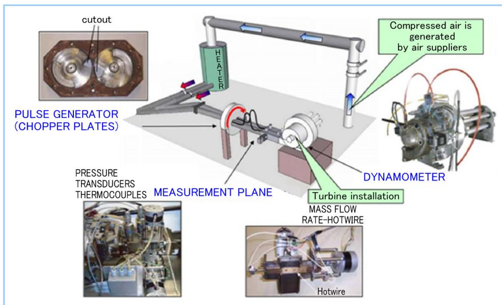
**Figure 2** Turbine pulsating flow test equipment at ICL,
