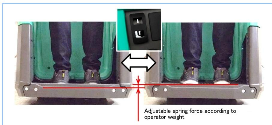
**Figure 10 Platform damper with spring force adjustment mechanism**
