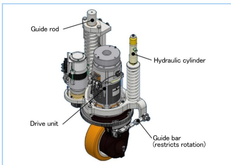
**Figure 6** Friction force system
