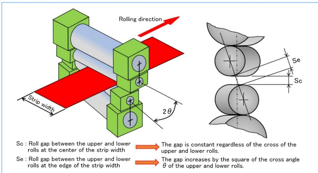
Figure 2 Principles of PC Mill
