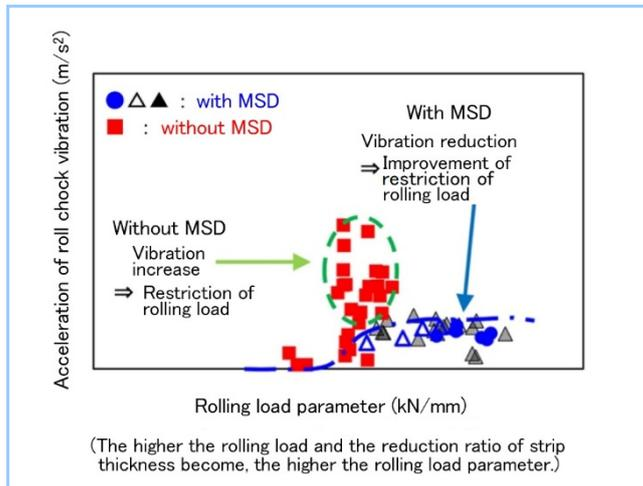
Figure 4 High load rolling by MSD
