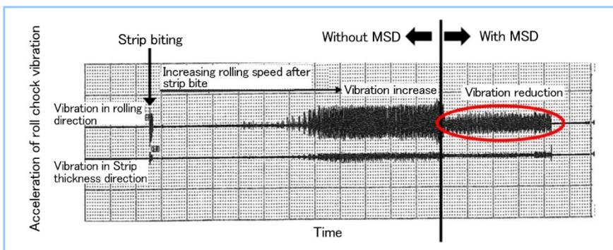
Figure 3 Reduction of mill vibration by MSD
