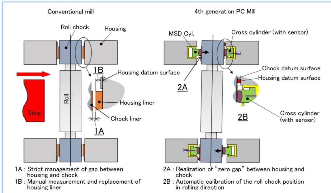
Figure 6 Labor saving and automation in liner management
