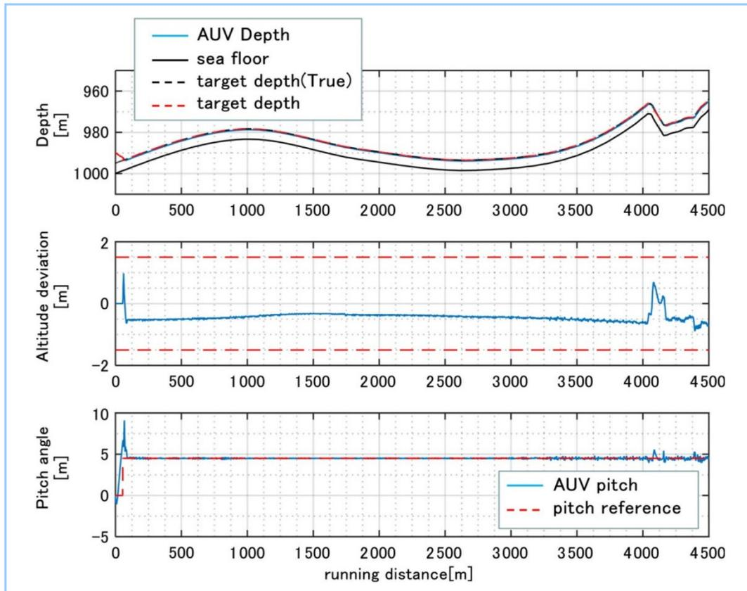
**Figure 6** Control results (above: depth, seabed topography and target trajectory; middle: altitude deviation; and below: pitch angle)
