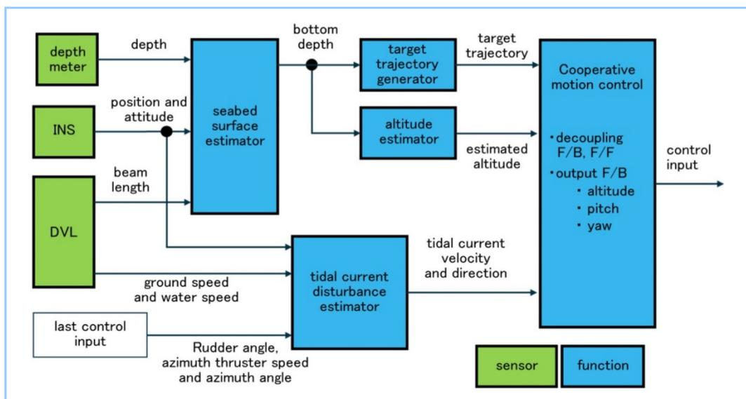
Figure 2 Functional configuration diagram of the autonomous control system
