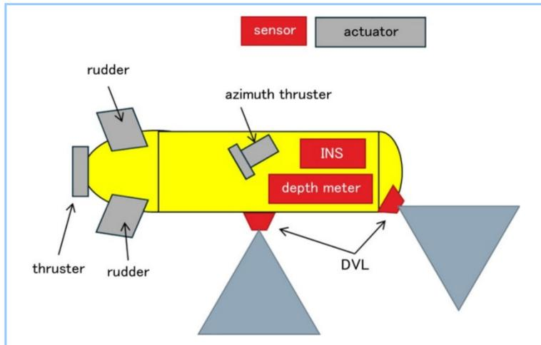
Figure 1 A schematic diagram of the AUV in this study
