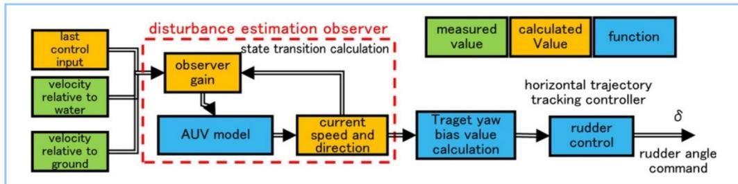
Figure 3 Tidal current estimation and direction control
