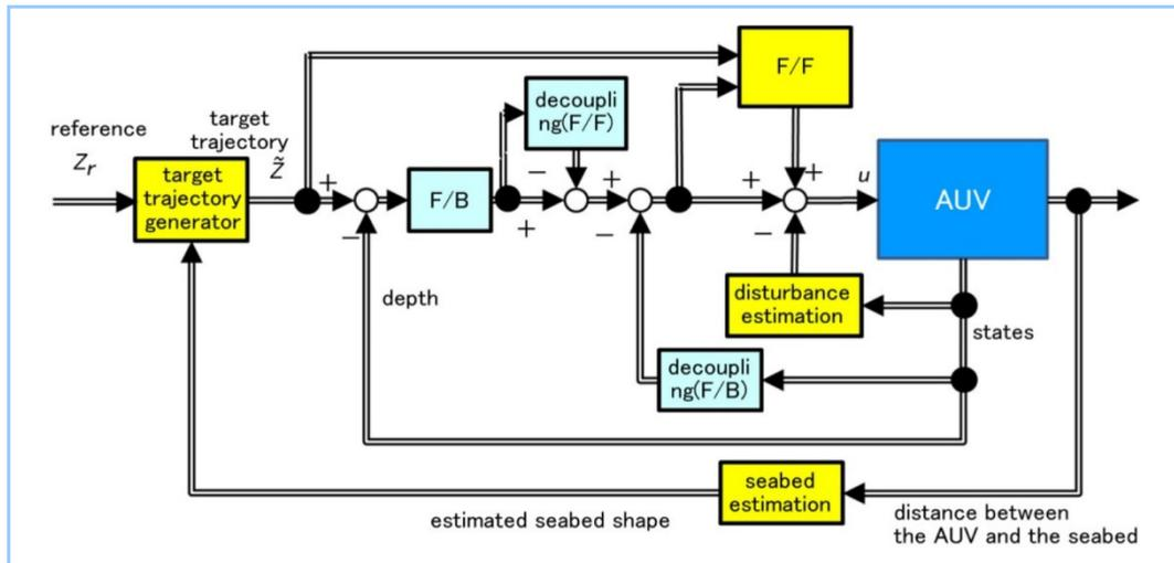
Figure 4 Block diagram of the autonomous control system
