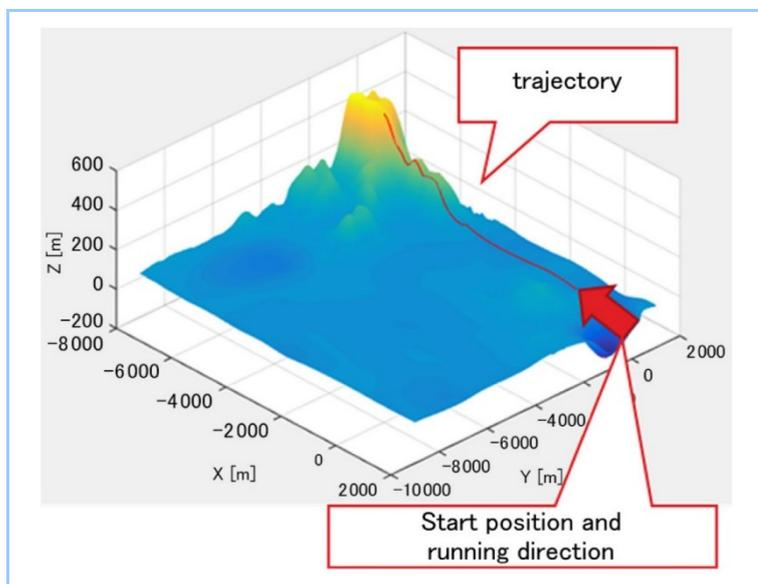
Figure 5 Seabed surface topography and the AUV's trajectory
