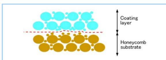
**Figure 1 Schematic diagram of bimodal coating technology using two-particle-size catalyst**
