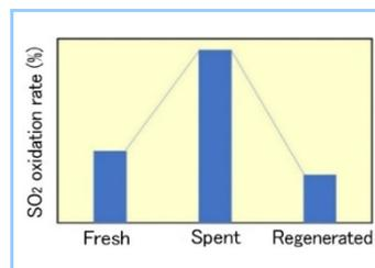
Figure 6 Comparison of SO<sub>2</sub> oxidation rate
