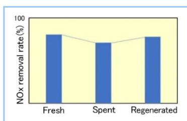
**Figure 2 Comparison of De-NO<sub>x</sub> performance**
