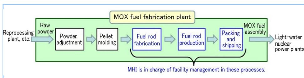
**Figure 4** MOX fuel fabrication process
