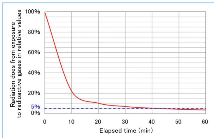
**Figure 2** Attenuation effect of noble gases and iodine
