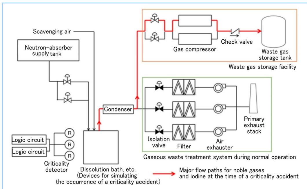
**Figure 3** System configuration of the waste gas storage facility
