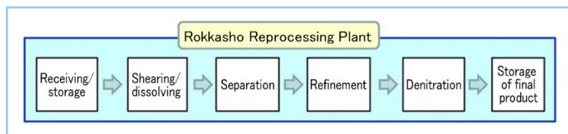
Figure 1 Overall process of spent fuel reprocessing
