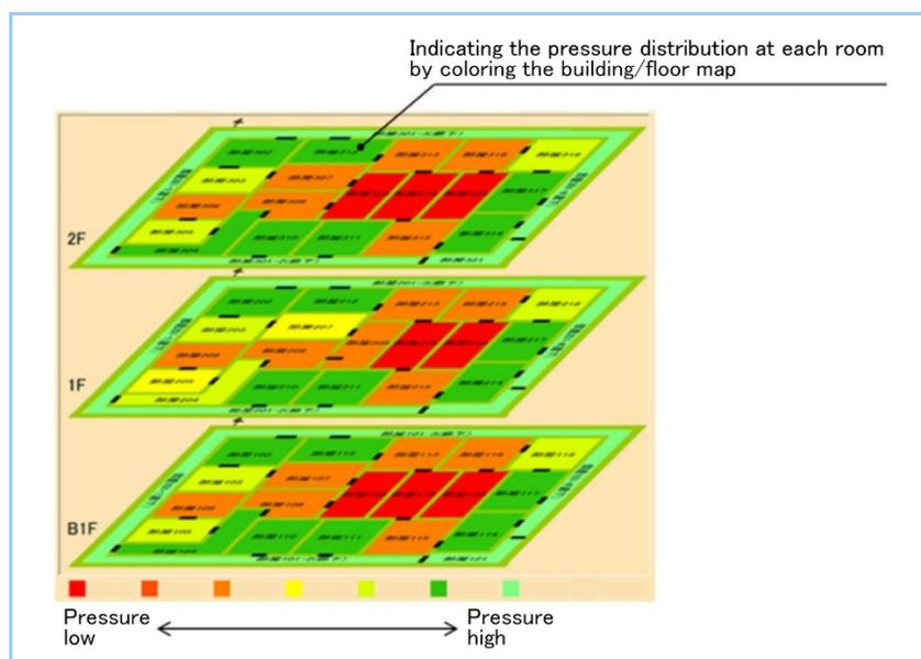
**Figure 5** Image of ventilation simulation tool in action \*
