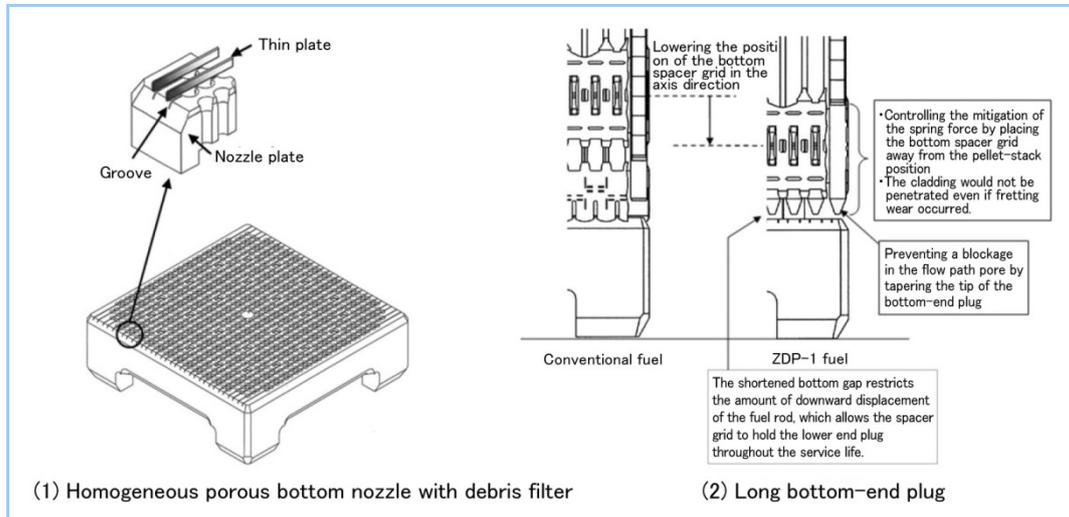
Figure 7 Measure for enhancing fretting wear resistance
