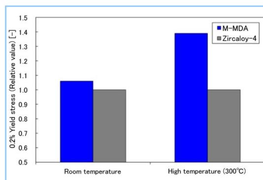
**Figure 4 Yield stress of sheet for spacer grid**
