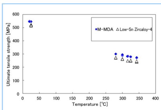
**Figure 3 Ultimate tensile strength of guide thimble**
