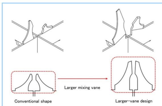
Figure 8 Comparison between 2 different mixing vane shapes of spacer grid
