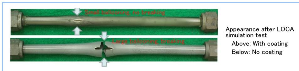
**Figure 9 Confirmed accident-tolerance effect**
