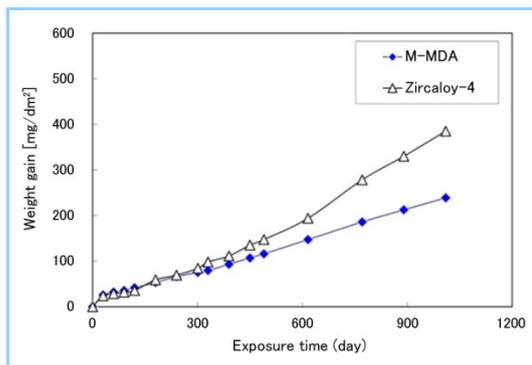
**Figure 2 Corrosion behavior of guide thimble**
