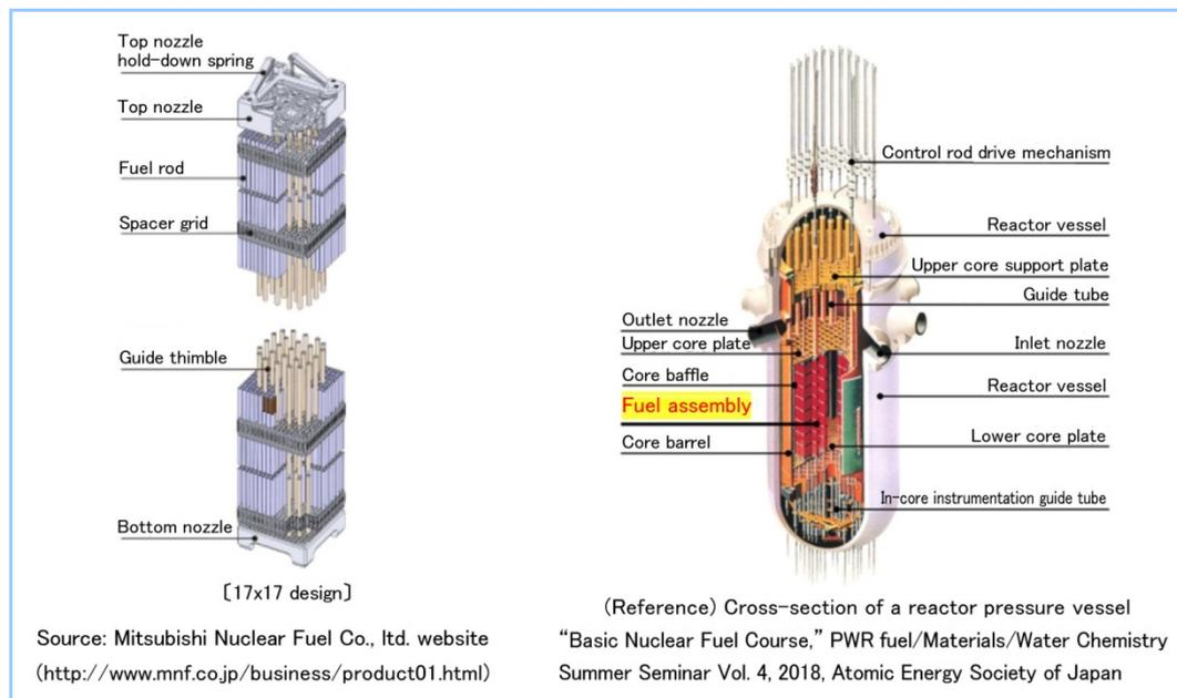
**Figure 1 Overview of fuel assembly for PWR**
