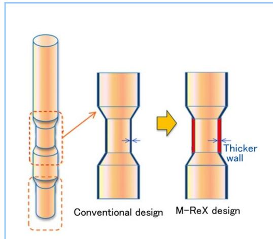
Figure 6 Measures for increasing margin in seismic resistance of guide thimble
