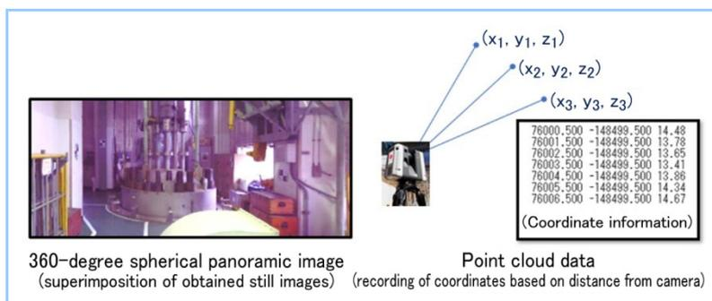
Figure 2 Image and data obtained by 3D laser scanner
