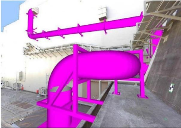
**Figure 4** Graphic representation of 3D-CAD data superimposed on point cloud panoramic data
