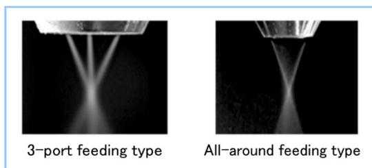
**Figure 3** Powder feeding nozzle
