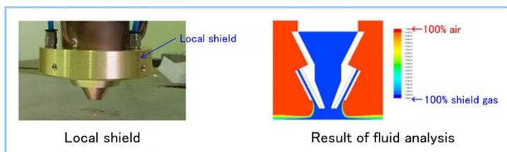
**Figure 4** Local shield and result of fluid analysis
