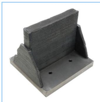
**Figure 9** Low thermal expansion alloy bracket
