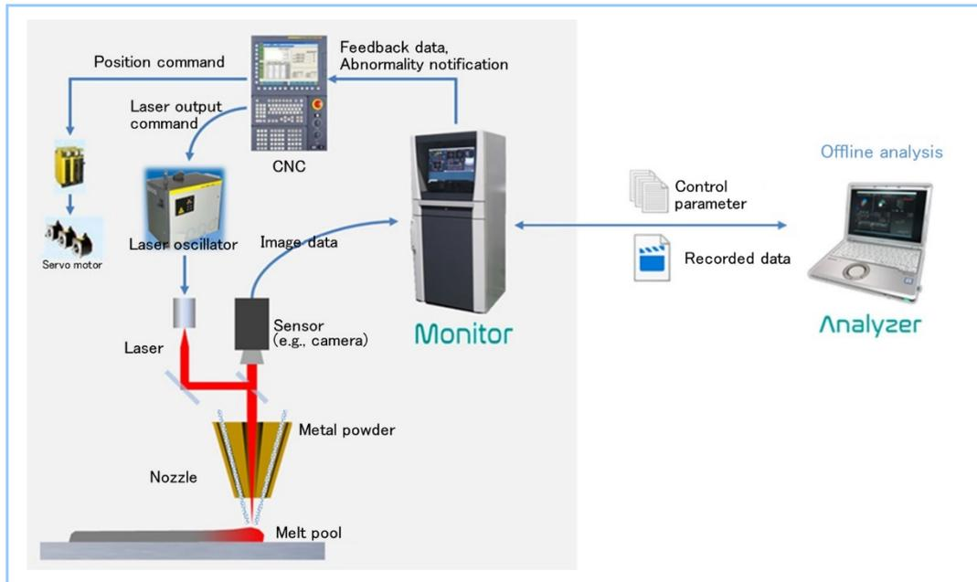
**Figure 5 Monitoring function system configuration**
