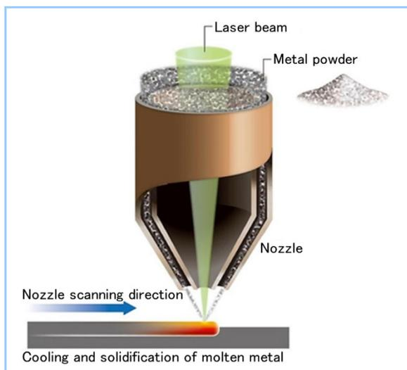
**Figure 1 Powder DED metal-based additive manufacturing method**
