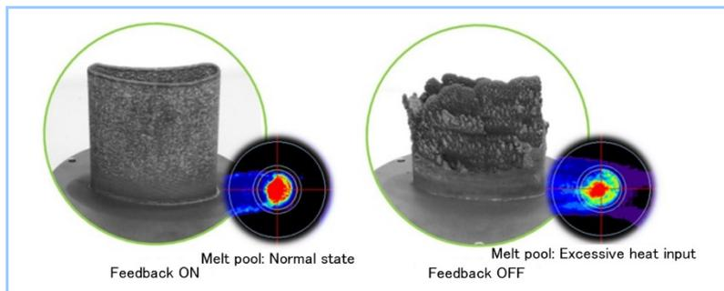
**Figure 6 Effect of monitoring feedback**
