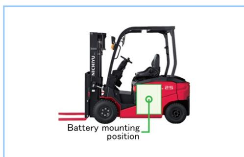
**Figure 4** Battery mounting position
