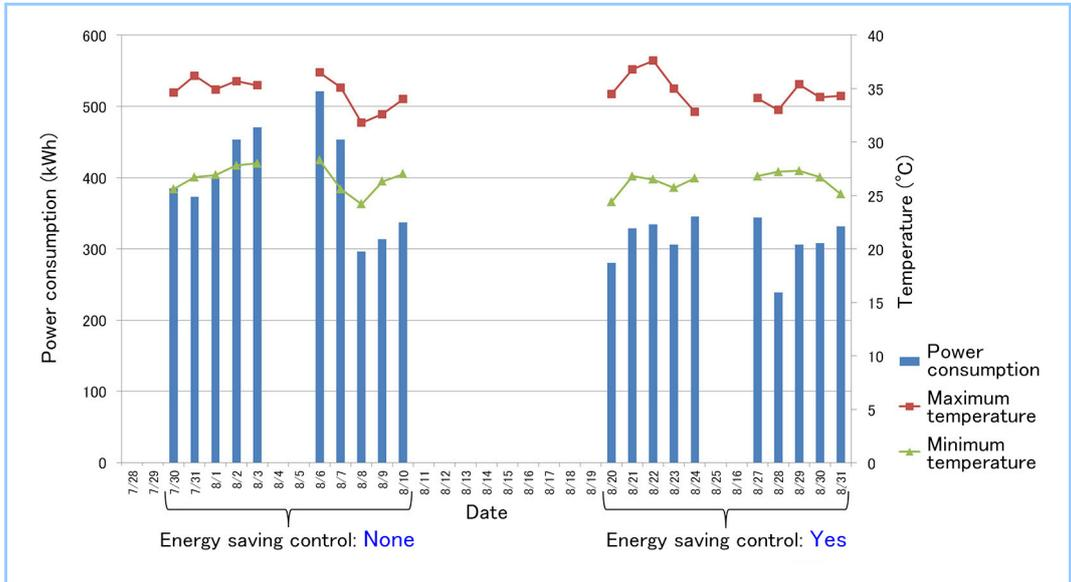
Figure 2 Energy saving effect through control of annual electric energy target
