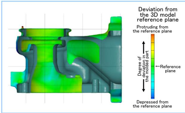
**Figure 6 Internal geometry measurement of the metal additively-manufactured turbine housing using X-ray CT**
