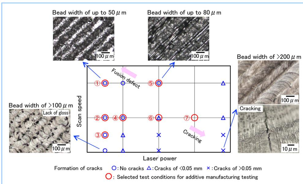
**Figure 2 Surface texture after laser beam irradiation of the casting material**
