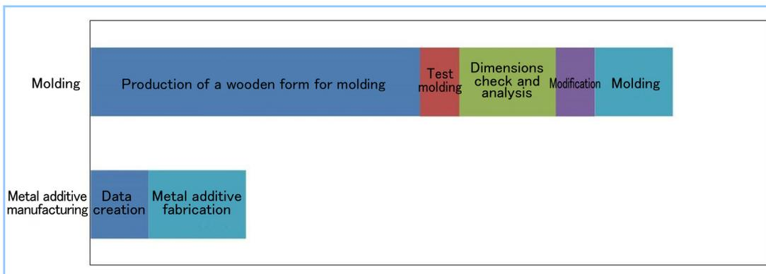
**Figure 7 Comparison of the molding and metal additive manufacturing processes in terms of the lead time required for prototyping a turbine housing**
