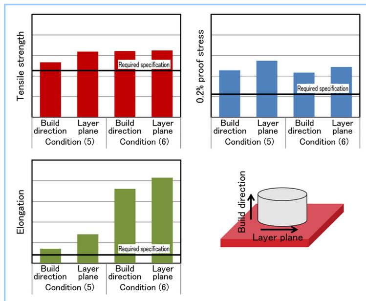
**Figure 5** Mechanical properties of the blocks built under conditions (5) and (6)
