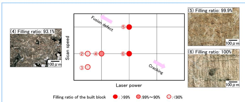
**Figure 4 Relationship between the filling ratio of the built block and the build conditions**
