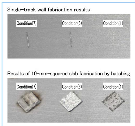
**Figure 3 Additive manufacturing testing results (building-up of 10 layers)**
