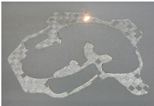
Photo of a turbocharger part being additively manufactured
