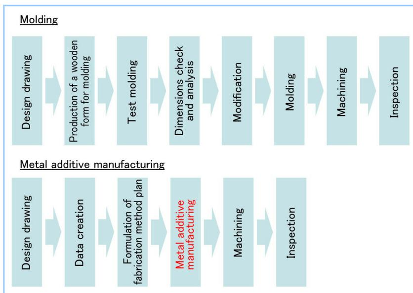
Figure 1 Flow charts for prototyping by molding and metal additive manufacturing
