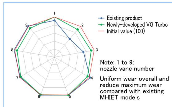
**Figure 14 Improvement of wear on drive part during engine endurance test**
