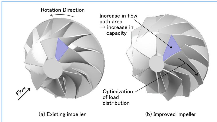
Figure 4 Improvement of compressor impeller
