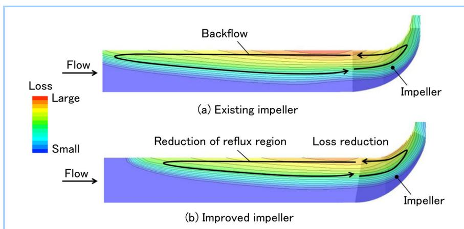
Figure 5 Loss Distribution at Maximum Torque Point
