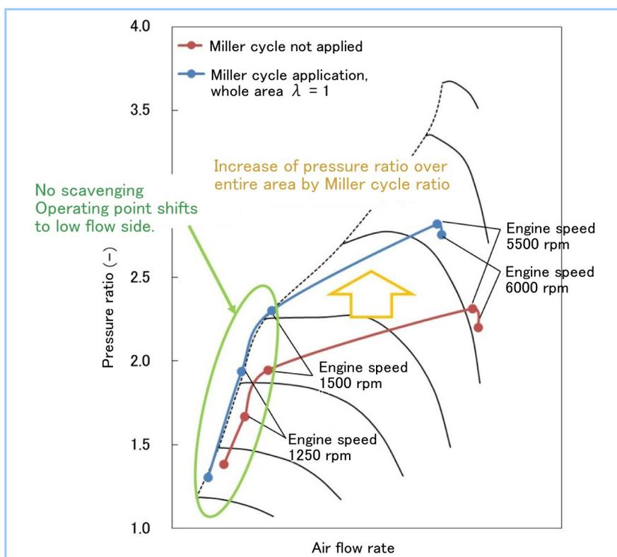
**Figure 2** Change in compressor operating point due to application of Miller cycle
