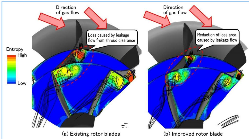
**Figure 11 Entropy distribution and flow line inside rotor blade**
