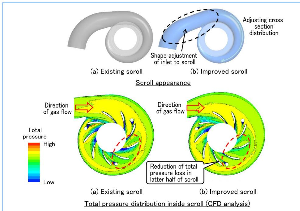
**Figure 9 Improved design of turbine scroll**
