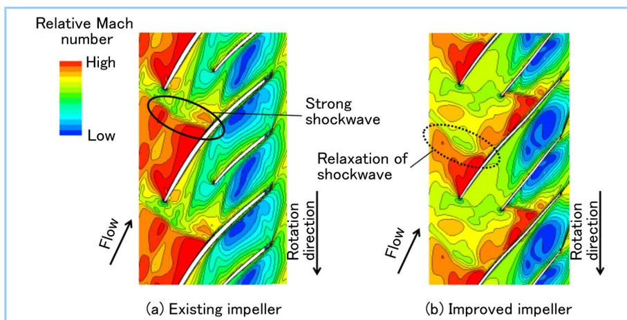
Figure 6 Relative Mach number distribution at maximum output point
