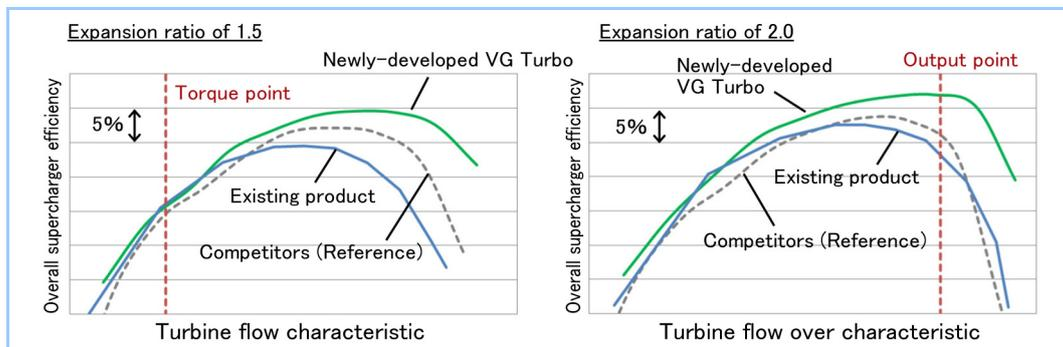
**Figure 12 Improvement of turbocharger efficiency by newly developed VG turbochargers**
