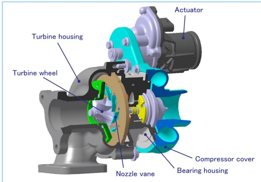
**Figure 1** Structure of VG turbochargers
