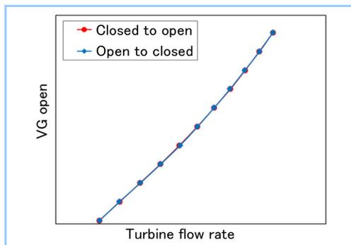
**Figure 13 Flow hysteresis evaluation test results**
