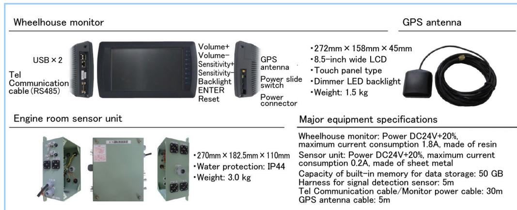
Figure 2 Overview and dimensions of the system
