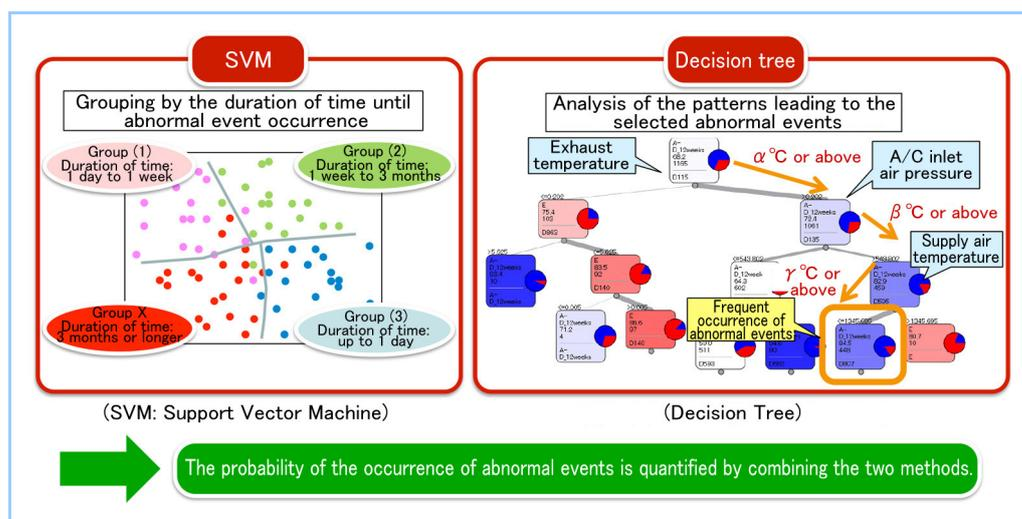
**Figure 5** Outline of developed data mining technique
