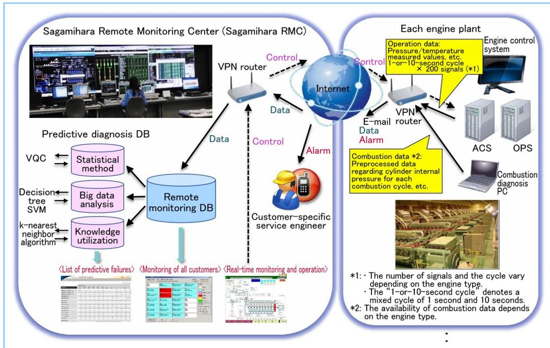
Figure 1 Configuration diagram of entire system
