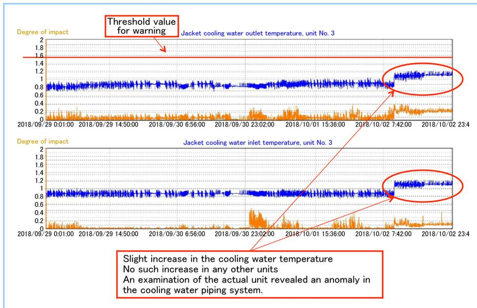
**Figure 3 Predictive failure report example 1**
