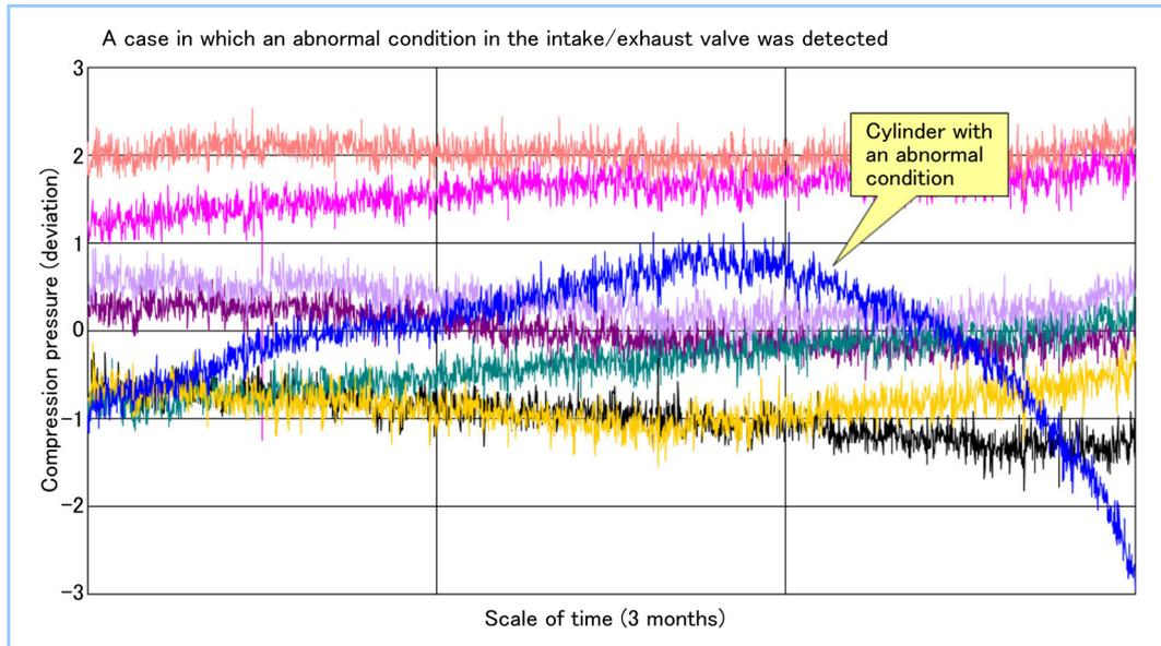
Figure 7 An example of detected abnormal conditions in the intake/exhaust valve
