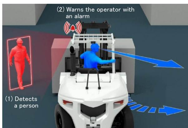
**Figure 1 Safe operation support using human detection system**
