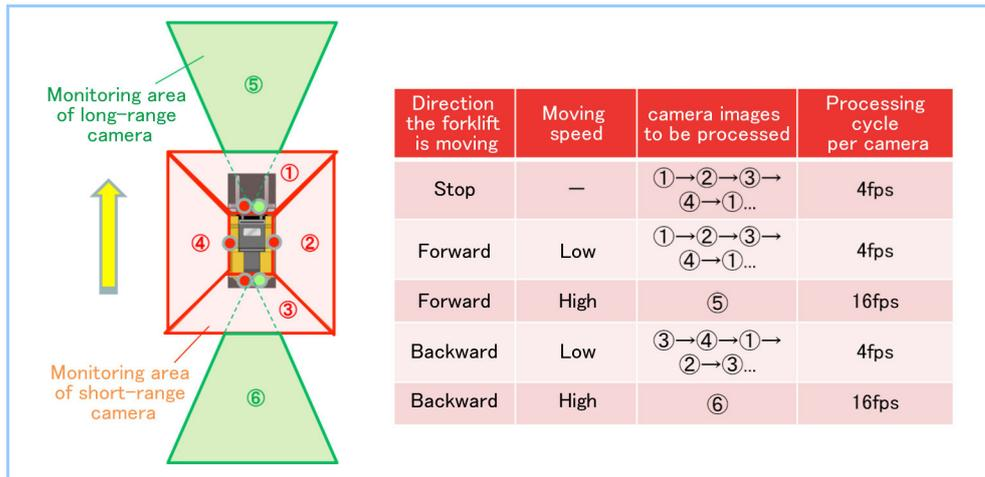
Figure 4 Automatic camera switching according to forklift conditions
