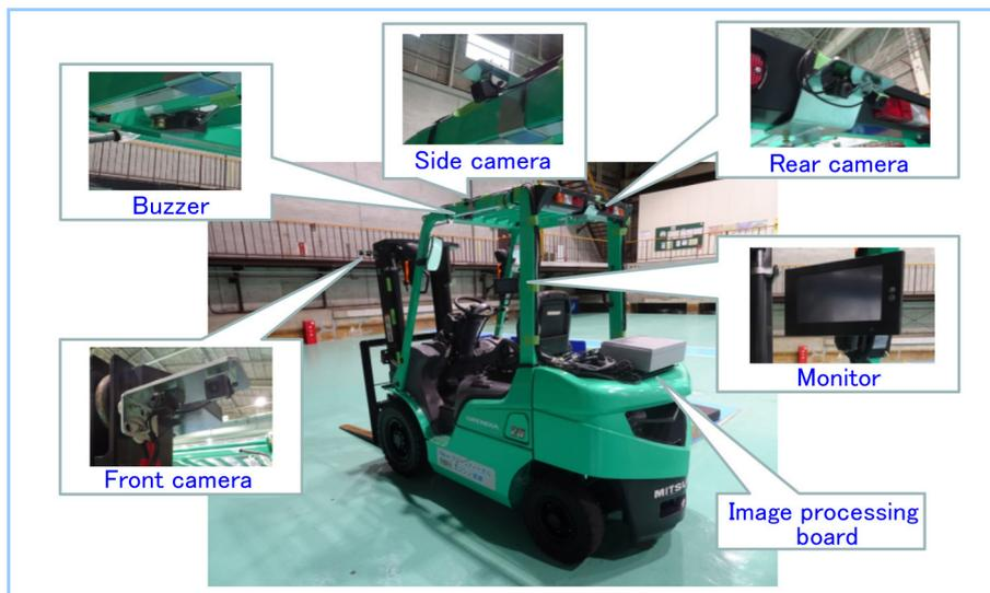
**Figure 3** Prototype human detection system for forklifts
