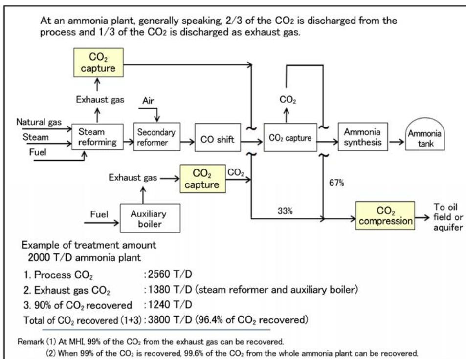
**Figure 2** CO<sub>2</sub> balance at an ammonia plant
