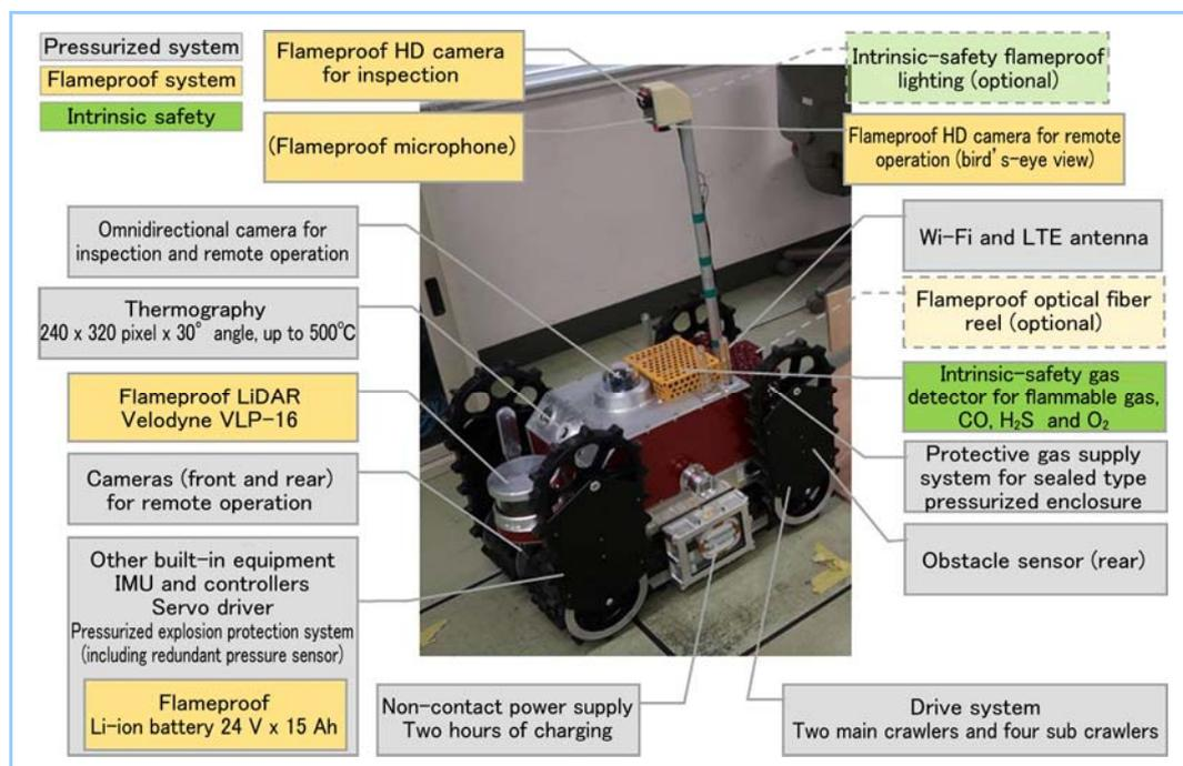
**Figure 2** Appearance and equipment configuration of robot
