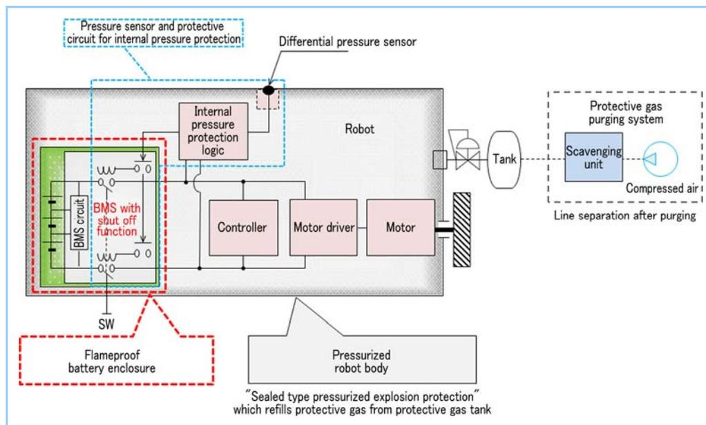
**Figure 3** Explosion protection structure of robot
