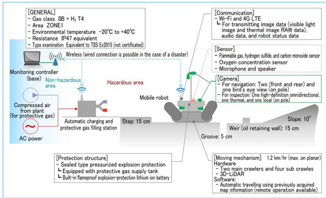
**Figure 1** Outline of system and specifications of explosion-proof autonomous robot
