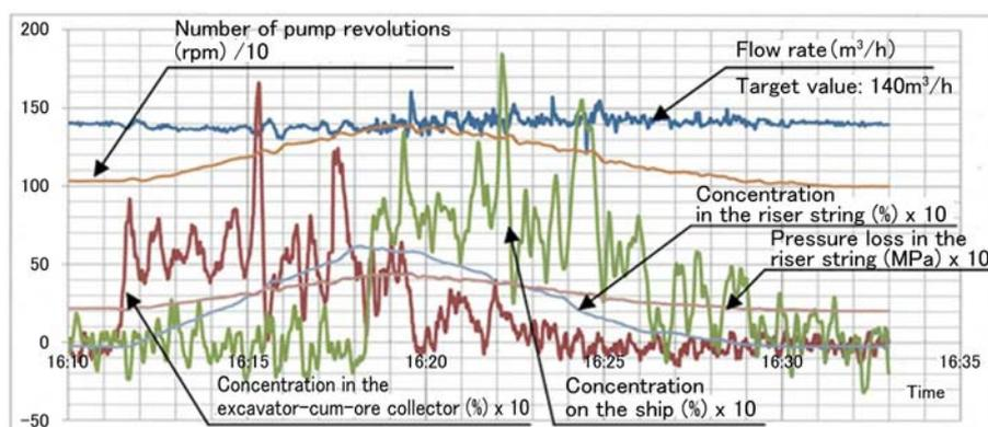
**Figure 8 Slurry ore lifting test and automatic flow rate control results**
