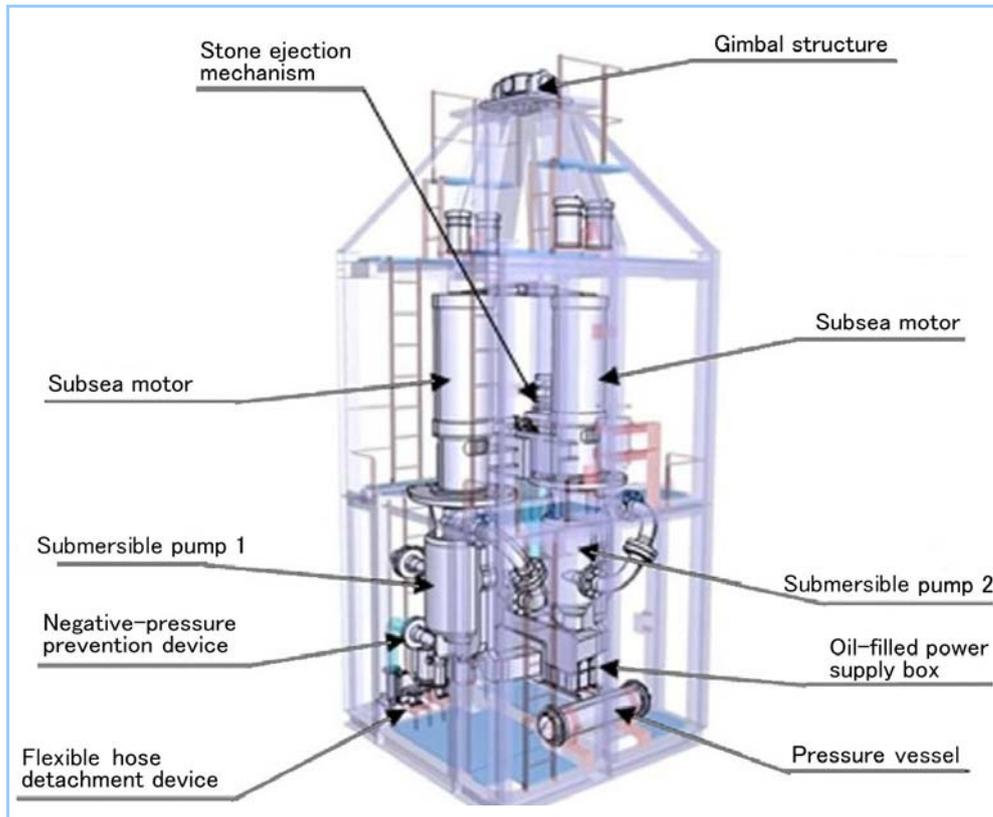
**Figure 5 Submersible pump unit configuration**
