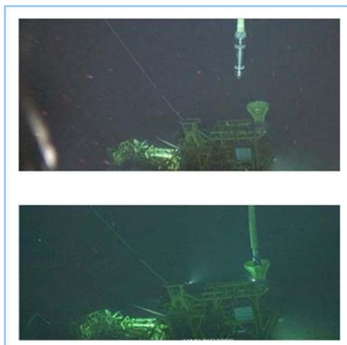
**Figure 7 Ore collecting test machine and the flexible hose before and after attachment**
