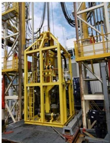
**Figure 6 Submersible pump unit**
