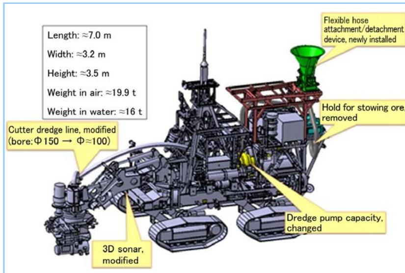
**Figure 2 Modifications made to the Ore collecting test machine**
