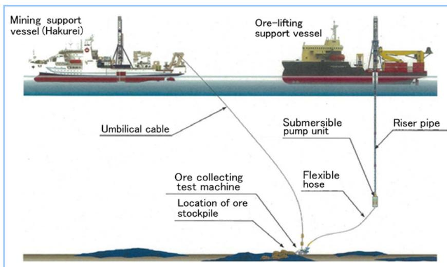
**Figure 1 Schematic diagram of the pilot test system**
