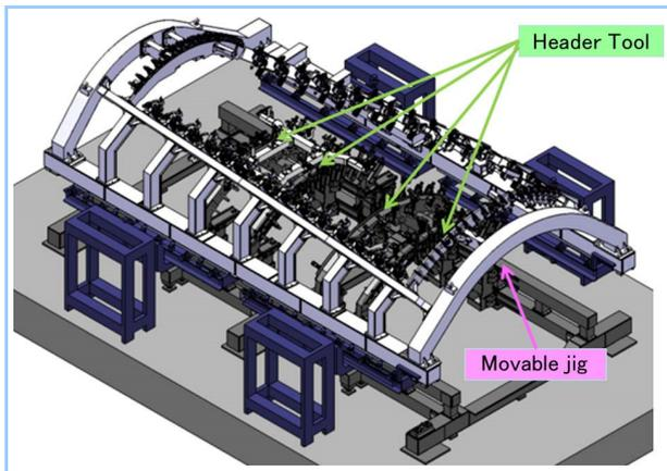
Figure 6 Header tool and movable jig
