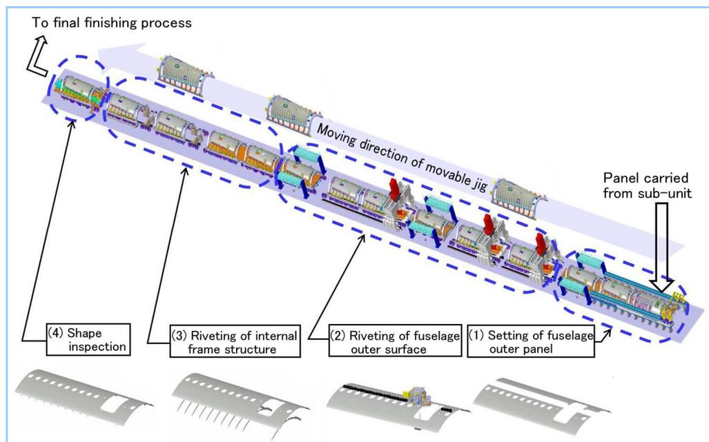
Figure 3 MPAL process schematic drawing
