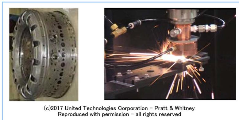
**Figure 6 Combustor and high-speed laser processing**
