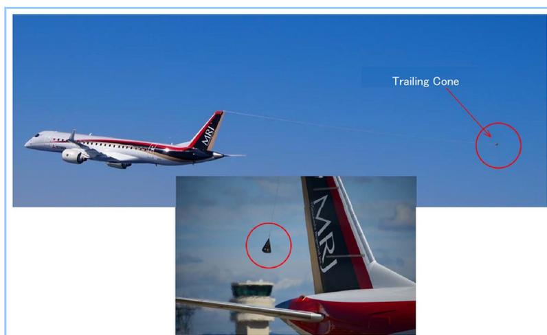
**Figure 4** Speed calibration test - trailing cone test
