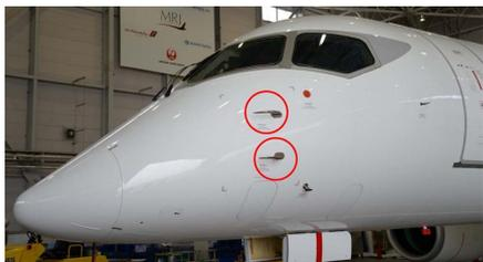
**Figure 3** Pitot tubes on MRJ
