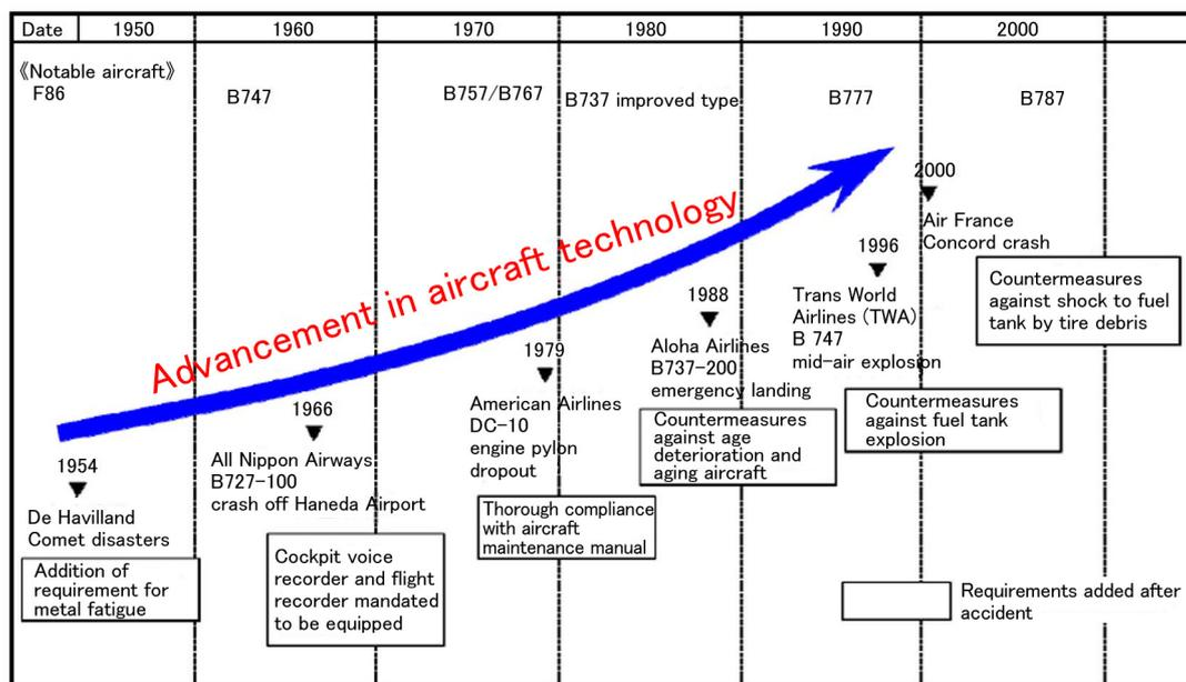
Figure 1 Technological progress of aircraft and history of safety requirements
