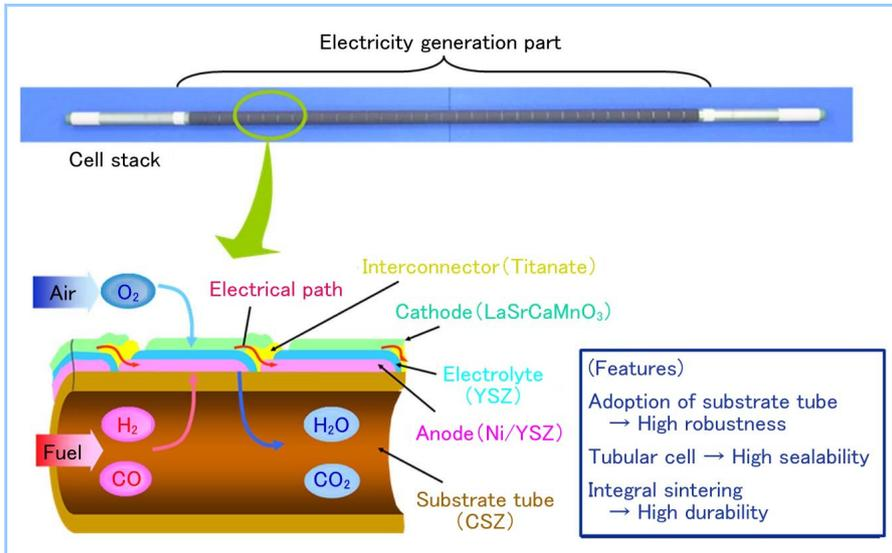
Figure 1 Structure of cell stack
