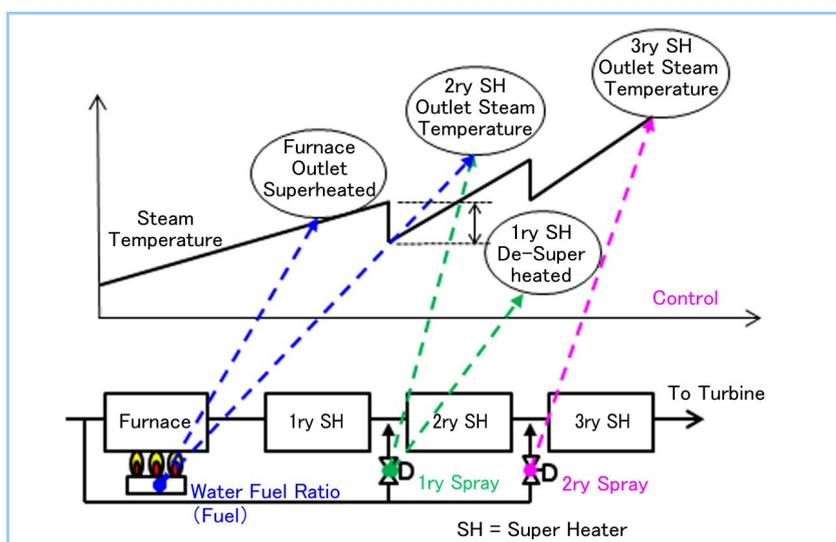
Figure 3 Conceptual diagram of steam temperature control (improved)
