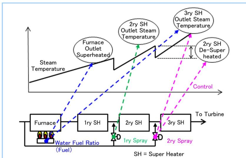
Figure 2 Conceptual diagram of steam temperature control (conventional)
