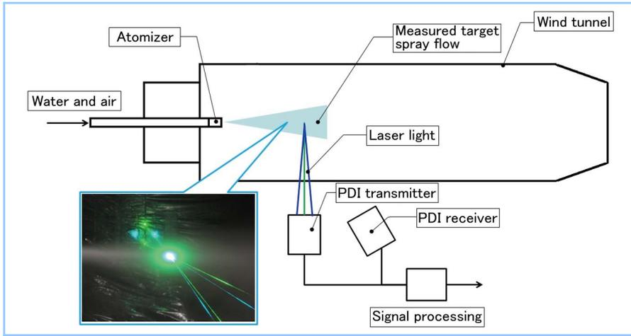
Figure 5 Measurement summary of water-air spray test
