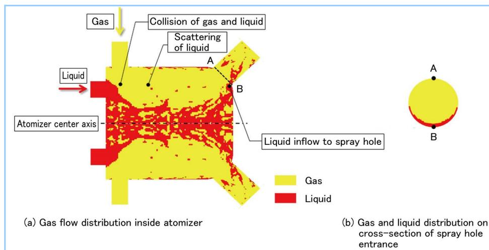
Figure 4 Internal flow analysis result of base atomizer
