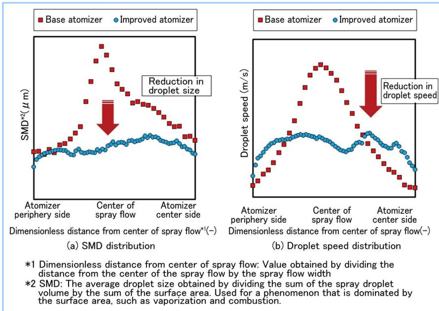
Figure 6 Spray test result
