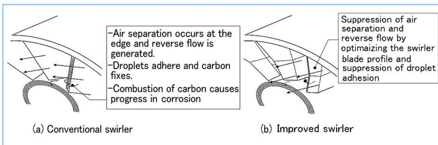
Figure 7 Combustion air flow around swirler
