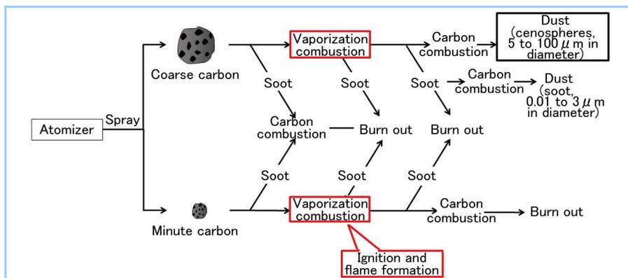
Figure 2 Combustion process of heavy oil fuel
