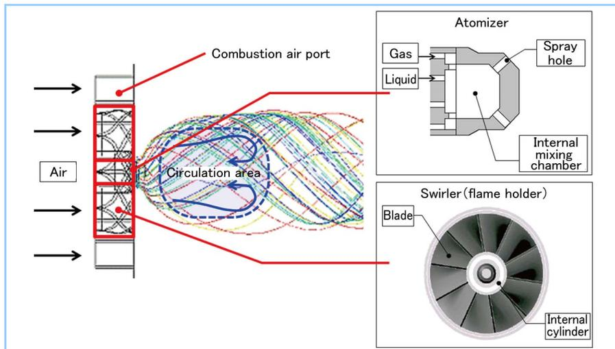
Figure 1 Basic configuration of heavy oil fired burner
