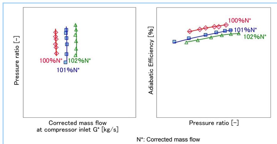
**Figure 4** Compressor overall performance
