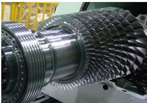
**Figure 1** Eight-stage compressor rotor
