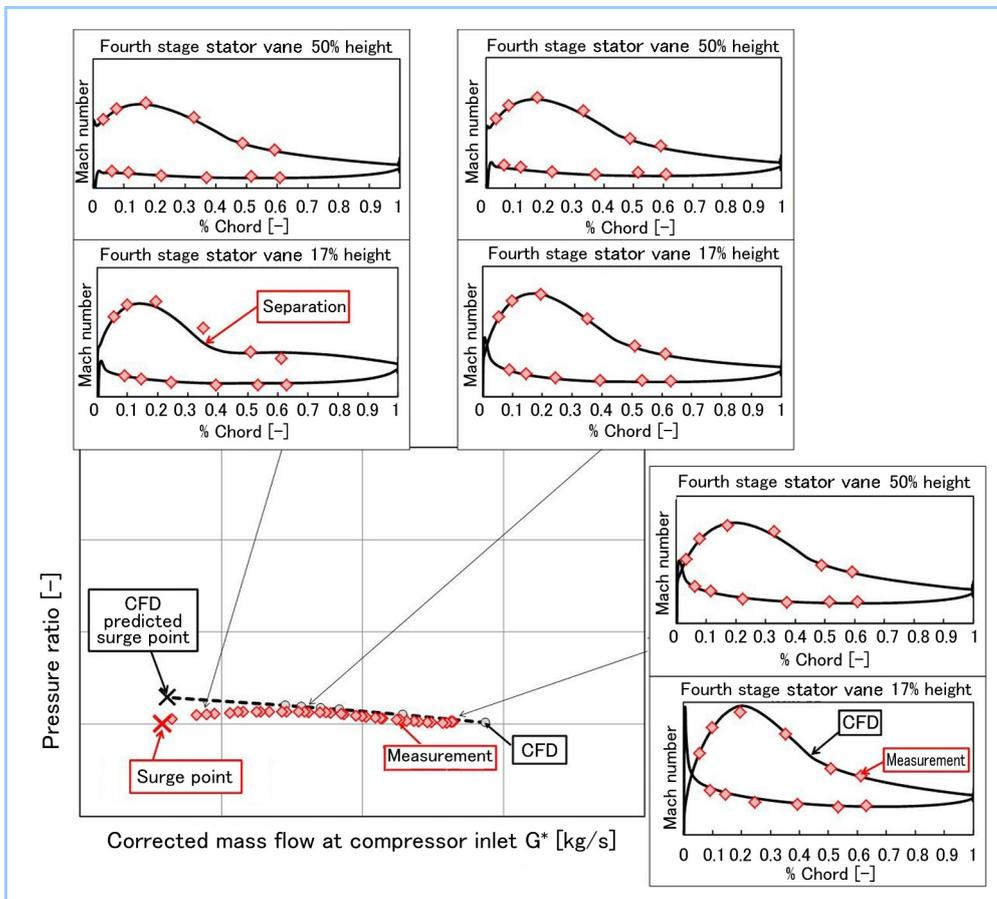
Figure 7 Compressor map and fourth stator surface static pressure at surge test
