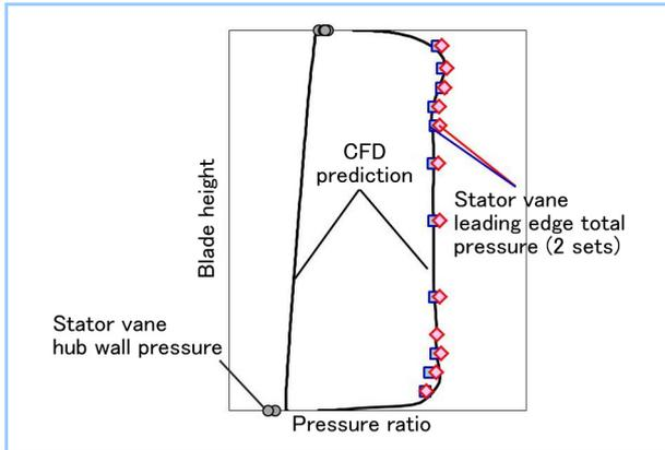
Figure 6 Leading edge total pressure and wall pressure of measurement blade made with 3D printer
