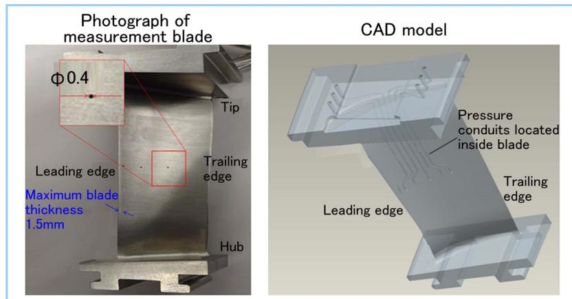
**Figure 3** Static pressure measurement blade made with a 3D printer (used as a set of two blades at three measurement points on each of the leading and trailing edge)
