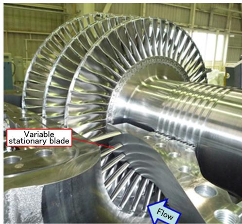
**Figure 2** Power recovery turbine
