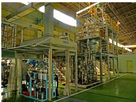
Figure 4 Biomass gasification and FT synthesis integration test facility
