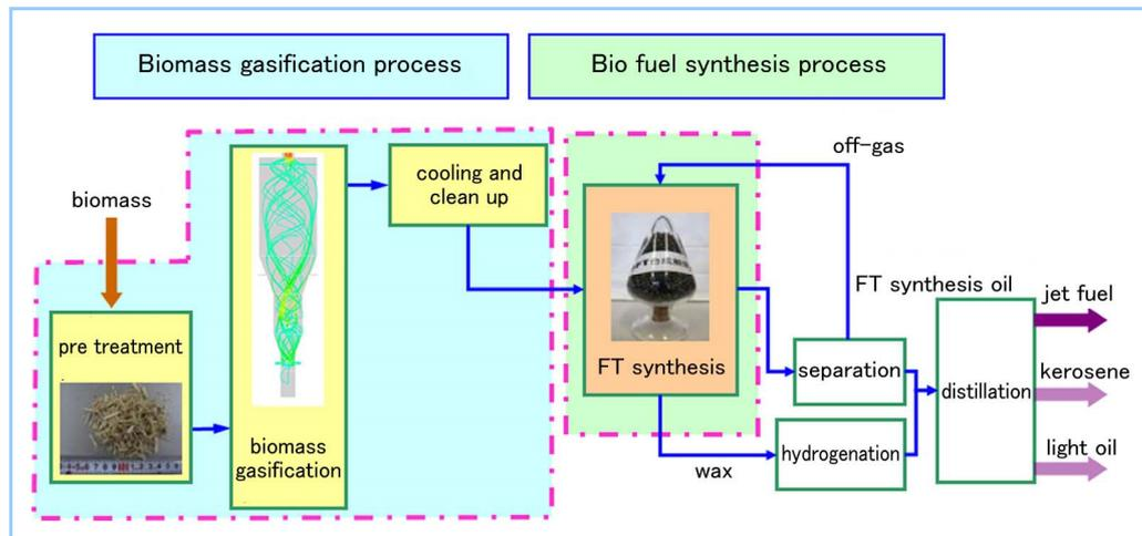
Figure 1 Bio jet fuel production process
