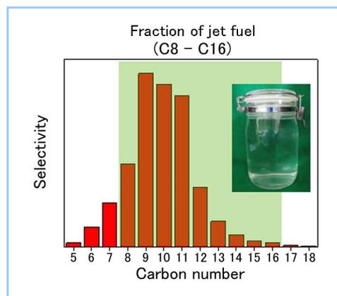
Figure 5 Carbon number distribution of FT synthesis oil
