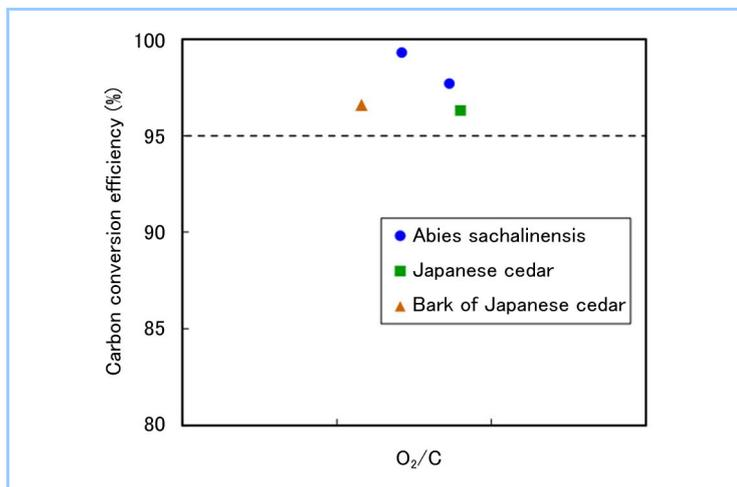
Figure 3 Carbon conversion rate of various types of biomass
