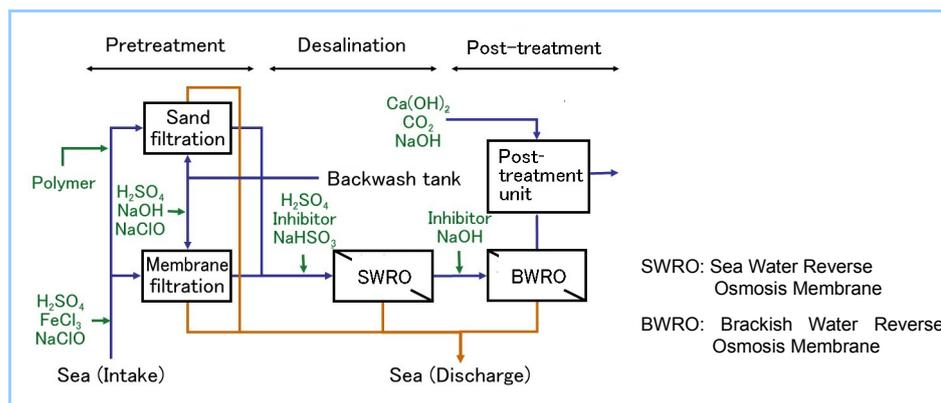
**Figure 1 Schematic flow diagram of SWRO desalination plant**
