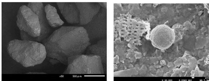
**Figure 4** SEM microphotograph of sand media filter
