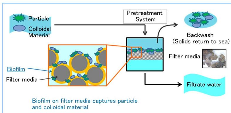
**Figure 5** Presumed chemical-free sand filtration mechanism
