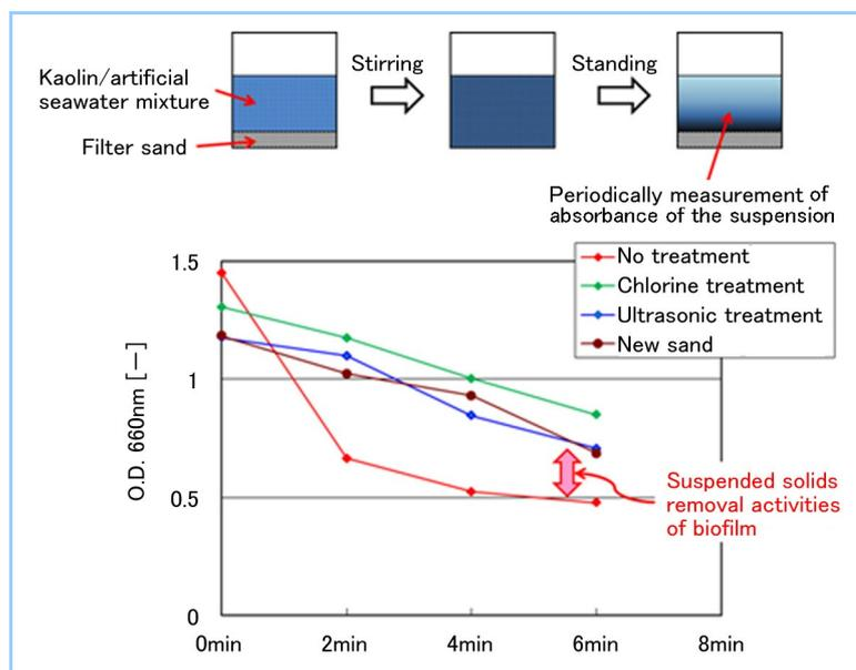
**Figure 6 Overview of laboratory-scale experiment and results of absorbance measurements**
