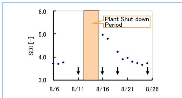
**Figure 2** Chronological changes in SDI of filtrate water from chemical-free pretreatment unit
