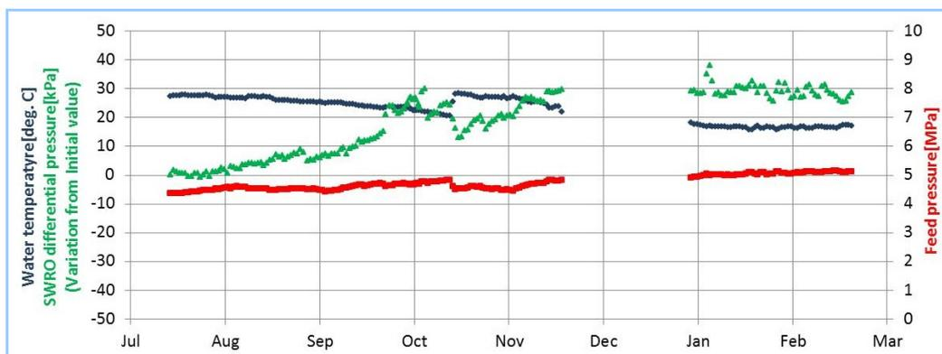
Figure 8 Chronological changes in feed pressure, SWRO differential pressure and water temperature
