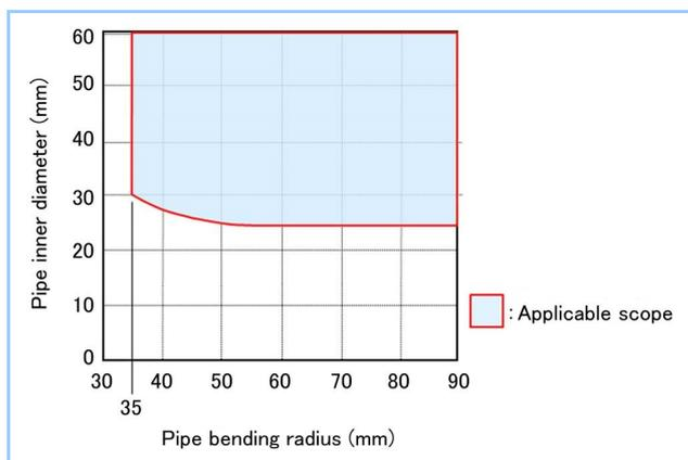
**Figure 9** Applicable conditions of tube inner diameter and tube bending radius
