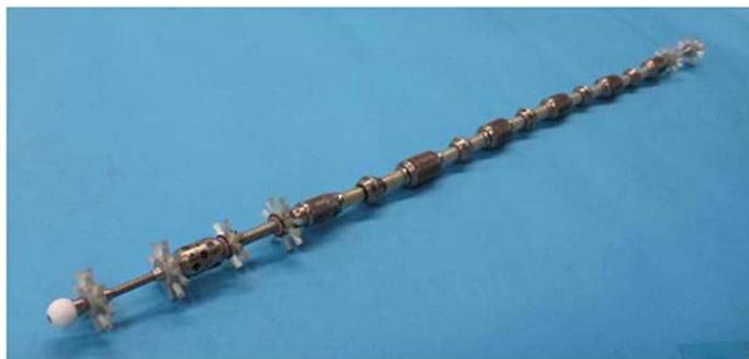
**Figure 2** Ultrasonic sensor for Cableless Inner UT system
