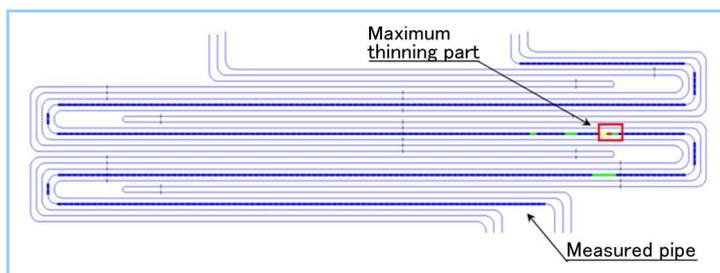
**Figure 8 Measurement results (panel diagram)**
