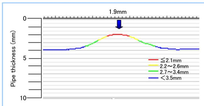
**Figure 7 Measurement results of maximum thinning part (cable-less inner UT system)**
