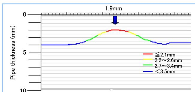
**Figure 6** Measurement results of maximum thinning part (conventional inner UT system)
