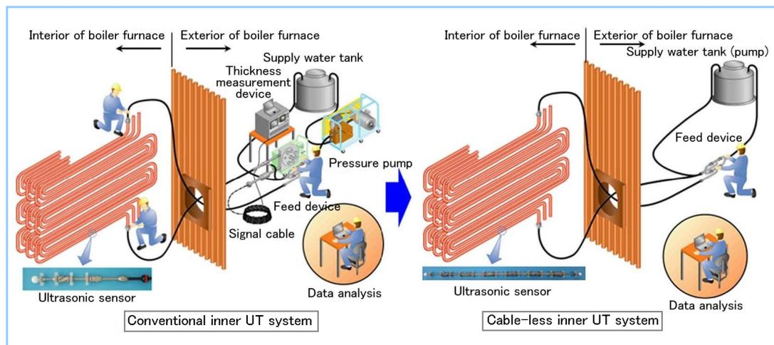
**Figure 1** Schematic diagram of conventional inner UT system and cable-less inner UT system
