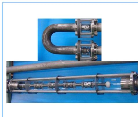
**Figure 5** Passage situation of sensor
