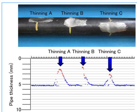
**Figure 4** Thickness measurement results (chart diagram)
