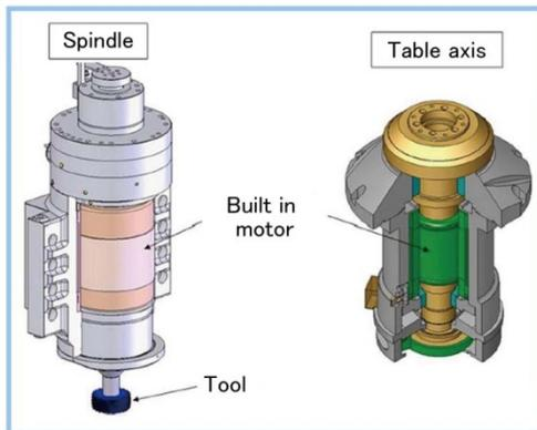
**Figure 7** Structure of spindle and table axis
