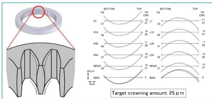
Figure 10 Tooth lead accuracy in crowning cutting
