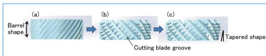
Figure 4 Barrel-shaped grinding wheel and super skiving cutter
