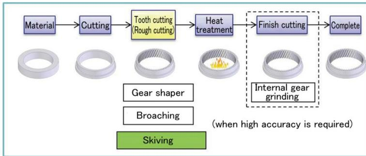
Figure 1 Manufacturing process of internal gear
