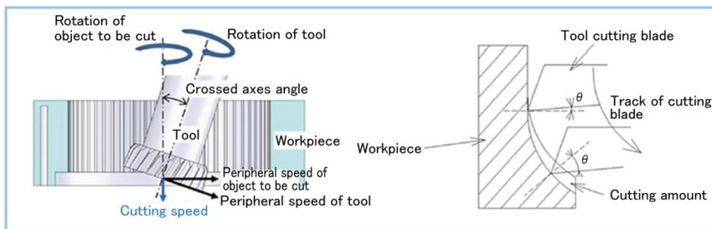
Figure 3 Principle of skiving cutting
