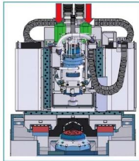
**Figure 6** Tandem control of feed axis in tooth lead direction
