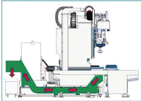
**Figure 5** Center trough structure
