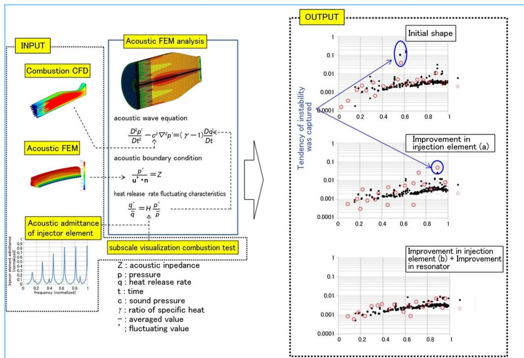
Figure 11 Combustion stability evaluation method (N- $\tau$  acoustic FEM analysis)
