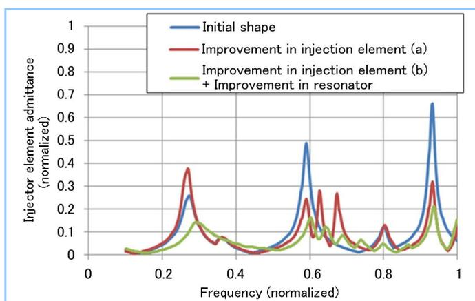
**Figure 8** Improvement in injector element acoustic admittance
