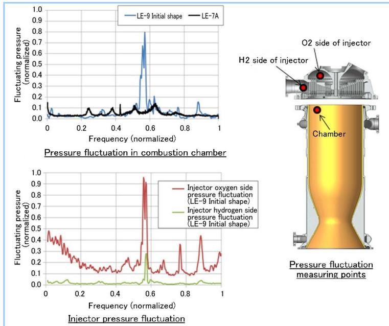
**Figure 6** Pressure fluctuation (initial shape)
