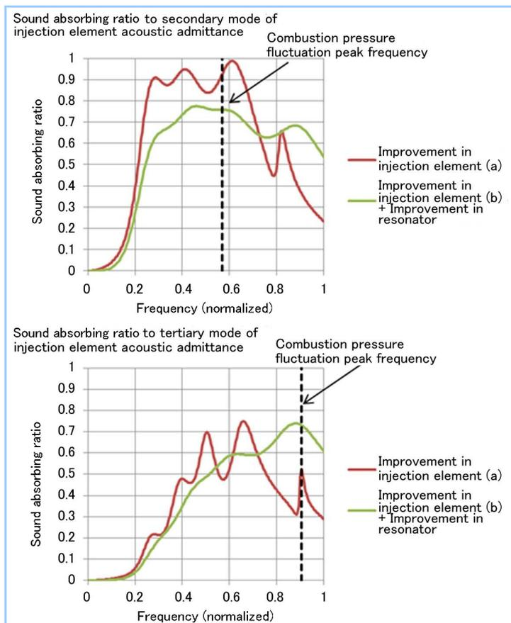
**Figure 9 Broadening of resonator**
