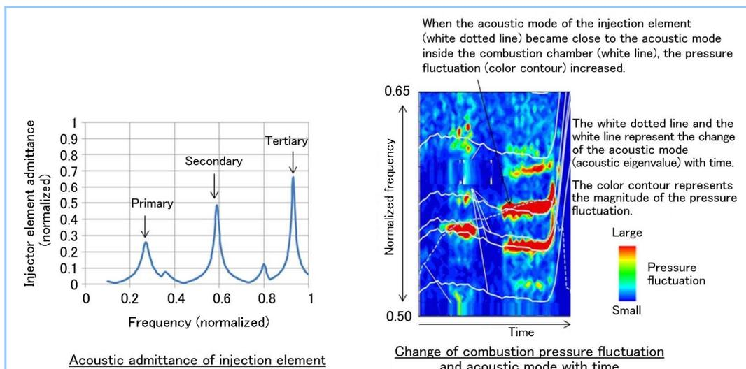
**Figure 7** Cause of unstable combustion (initial shape)
