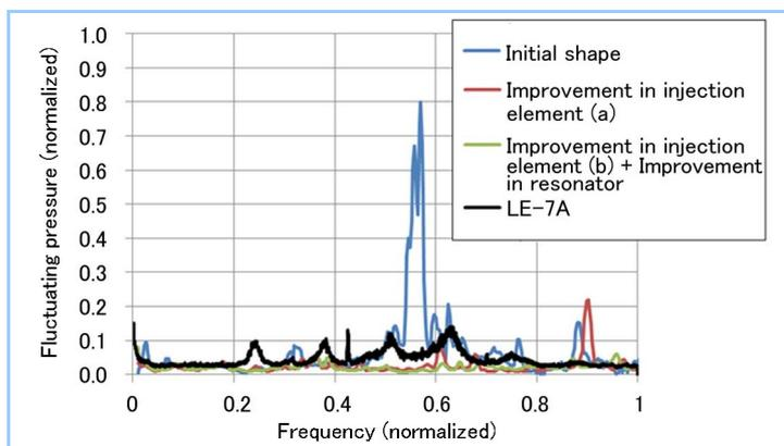
**Figure 10 Verification results of improvement in combustion stability**
