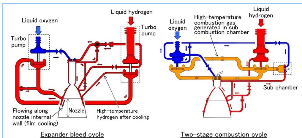
Figure 2 Engine cycle schematic view
