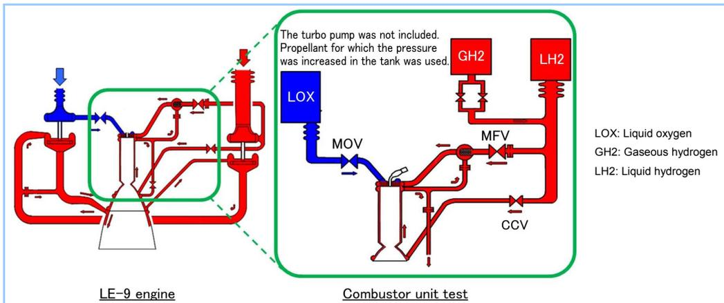
**Figure 3 Combustor unit test diagram**
