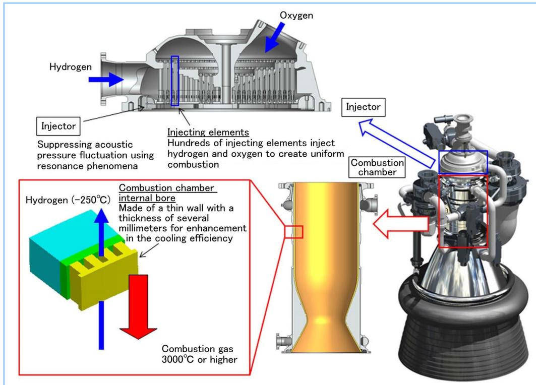
Figure 1 Structure of injector and combustion chamber
