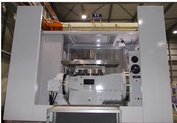
**Figure 2** 5-axis machining using rotating 2-axis table
