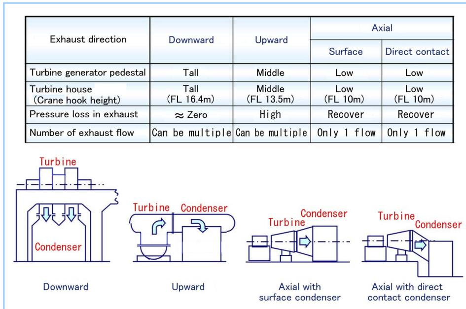
**Figure 5 Comparison of Turbine Exhaust Direction**
