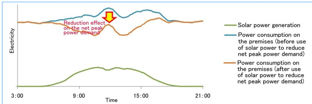
**Figure 3** Reduction effect on the net peak power demand resulting from solar power generation
