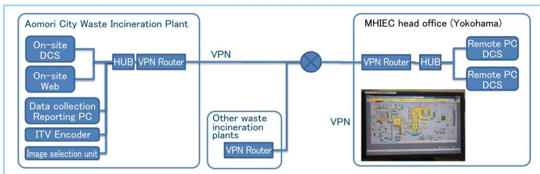
**Figure 4** Remote monitoring system
