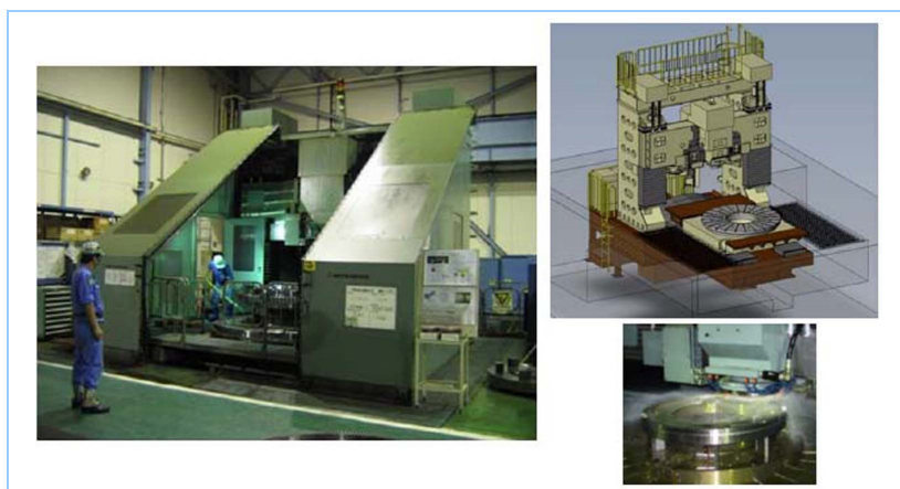
Figure 3 Disk coupling grinder and state of grinding (lower right)
