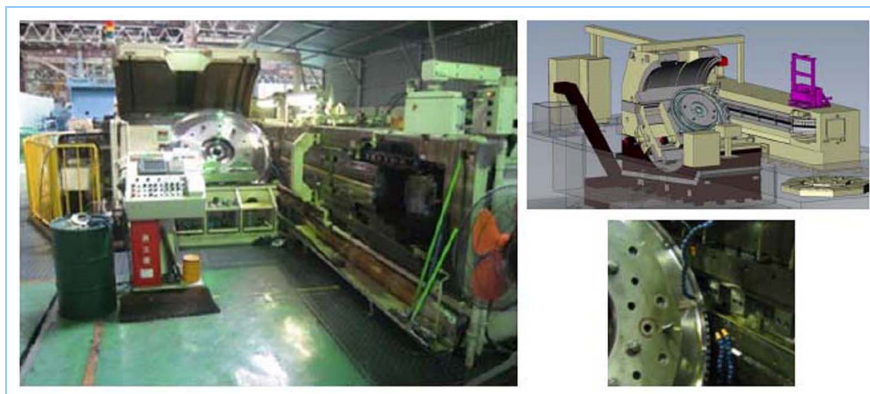
Figure 2 Chain broaching machine for gas turbine rotor disk processing, and state of broaching (lower right)
