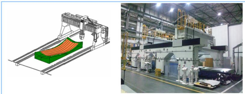
**Figure 3** Fuselage skin processing machine
