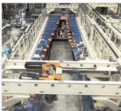
Figure 1 Main wing panel perforating machine
