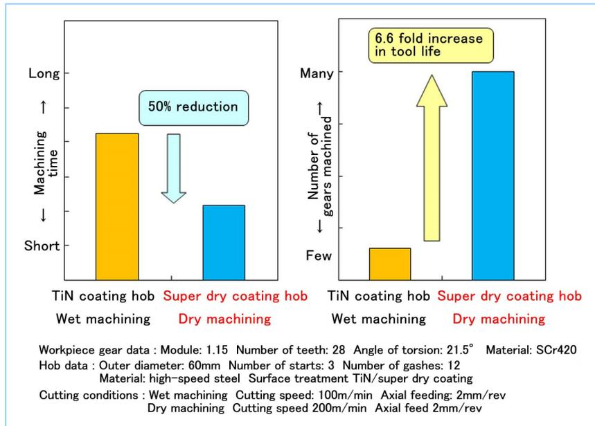
Figure 1 Example of dry gear machining with super dry coating hob
