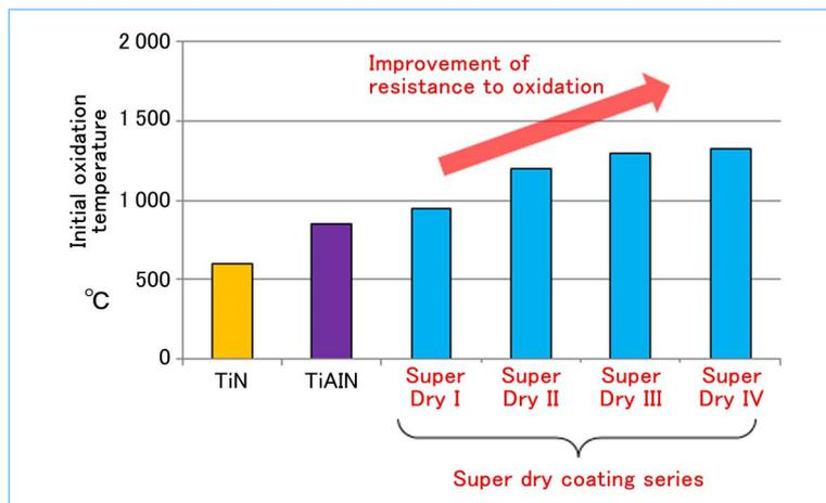
Figure 2 Initial oxidation temperature of super dry coating
