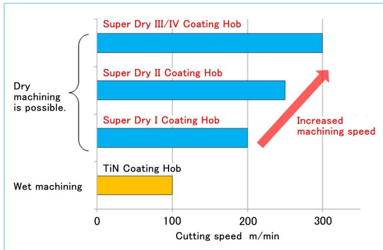
**Figure 3 Roughly estimated speed of gear machining using each super dry coating hob**
