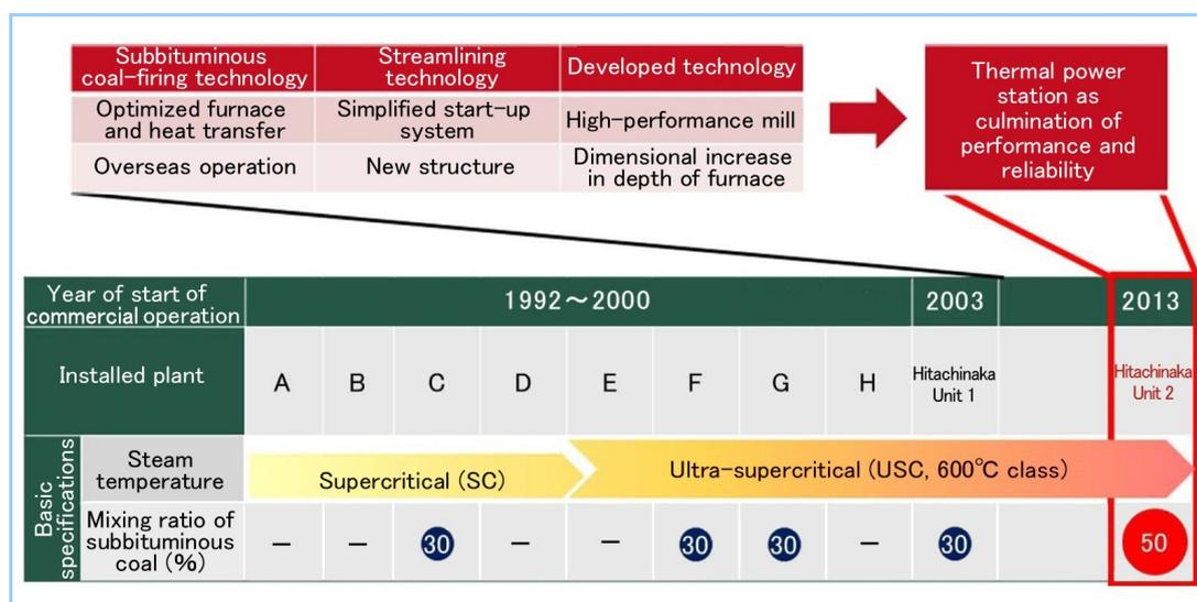
Figure 1 Upgrades of boiler basic specifications
